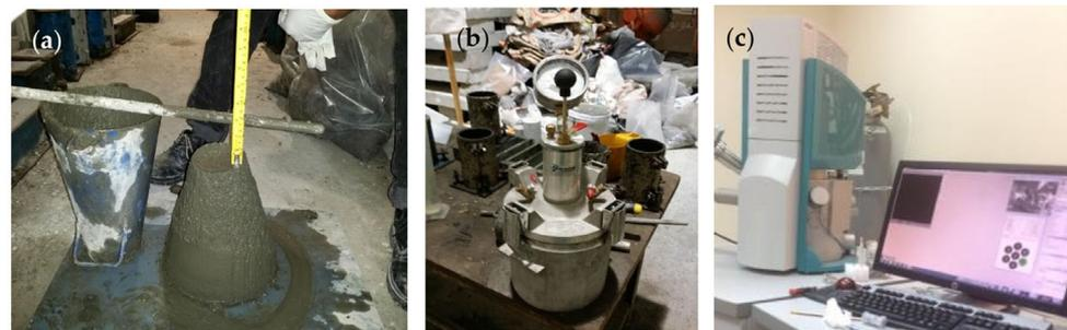
**Figure 4.** (a) Slump test. (b) Air content test. (c) SEM analysis.
