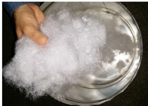
**Figure 2.** PE fibers treated with high-pressure air.
