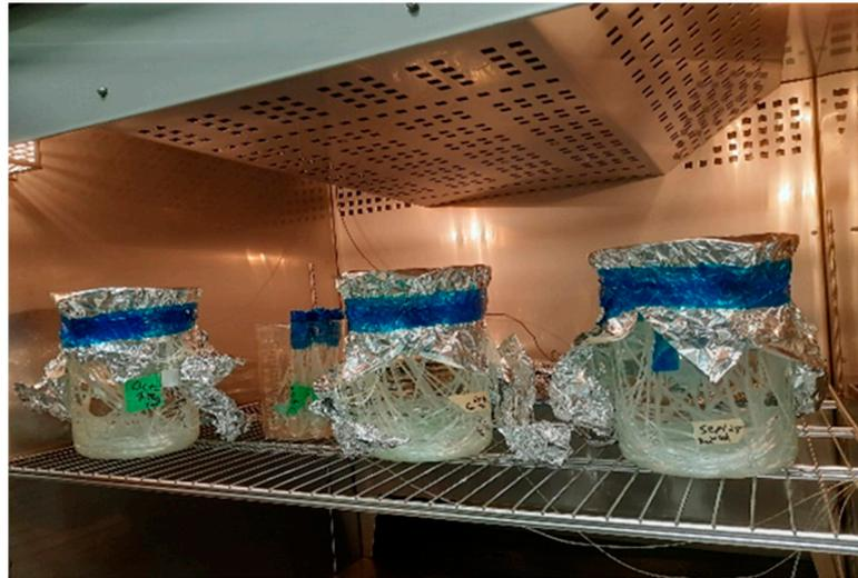
**Figure 1.** Aging of fiber samples inside oven.
