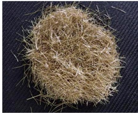
**Figure 2.** Golden-colored steel fiber was used in the experiment [22].**Table 2.** The result of the properties test of NSC, UHPC/UHPFRC, fiber, and steel bar.
