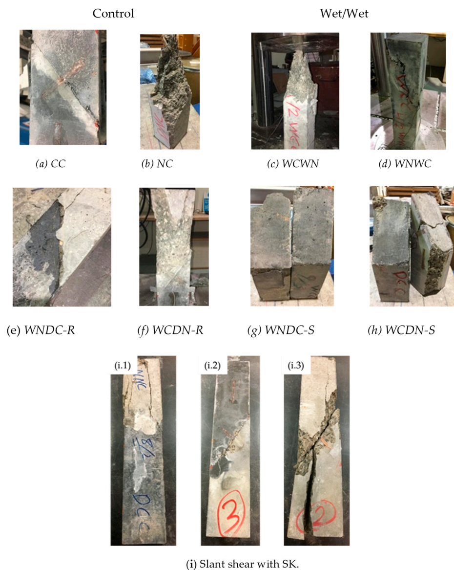
Figure 10. (a–h) General failure modes for slant shear samples. (i) Slant shear with SK surface preparation failure modes for (i.1) crushing failure, (i.2) bond failure, and (i.3) combination of both.
