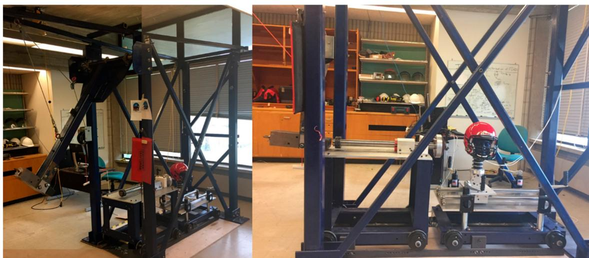
**Figure 3.** Pendulum based linear impactor with a magnesium head.
