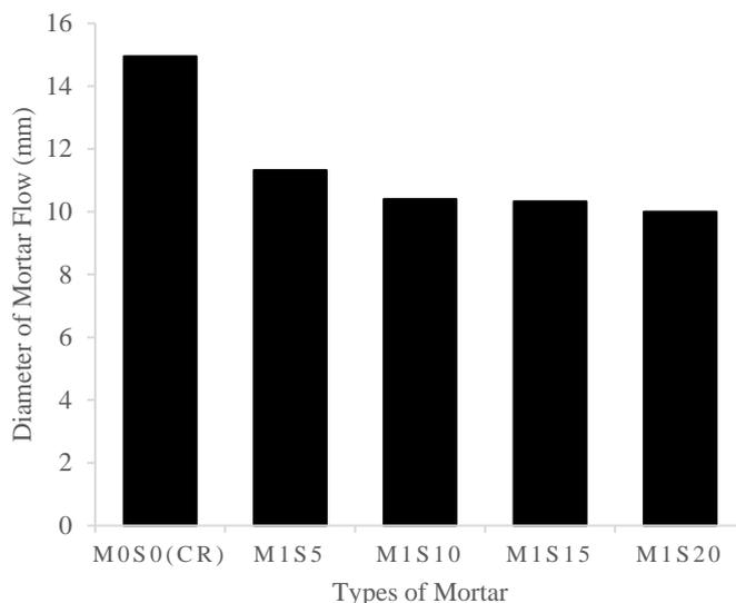
Figure 8. Effects of SF content on the workability of mortars containing 1% SDPMFs.
