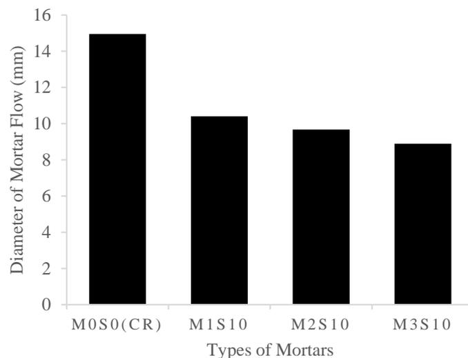
**Figure 7.** Effects of SDPMF content and 10% SF on the workability.
