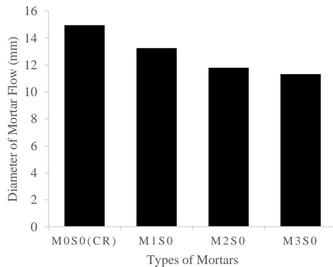
**Figure 6.** Effects of SDPMF content on the workability.
