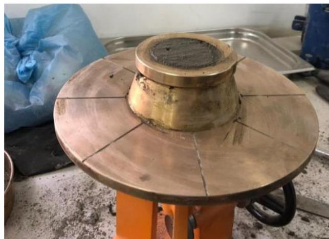
**Figure 5.** Workability test.
