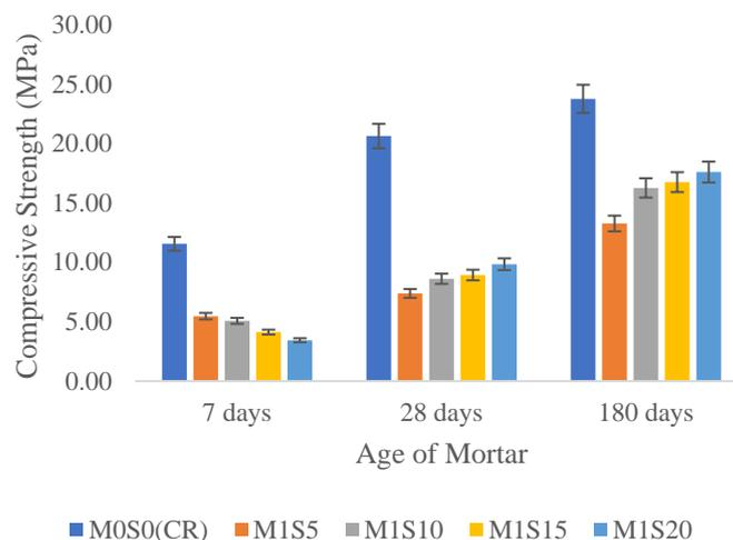
**Figure 12.** Effects of SF content on the compressive strength of 1% SDPMF mortars.
