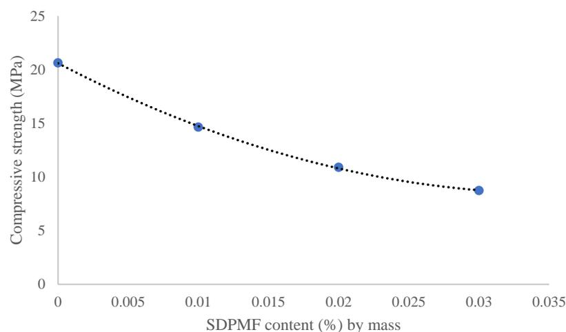
**Figure 10.** Best fit curve of SDPMF mortars' compressive strength.
