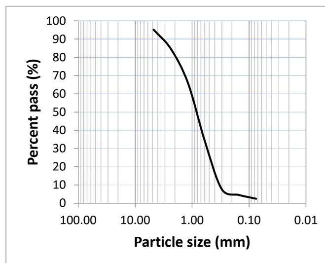
Figure 1. Particle size distribution of the used sand [23].
