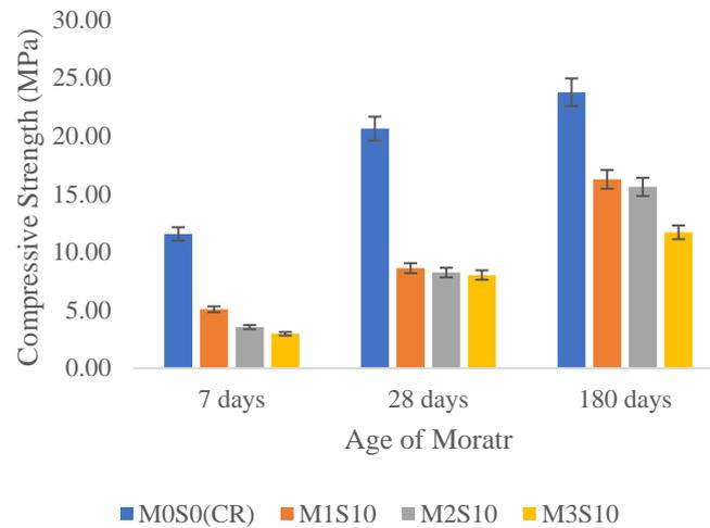
**Figure 11.** Effects of SDPMF content and 10% SF on mortars’ compressive strengths.
