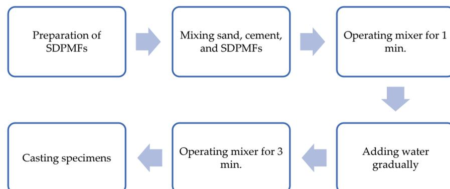
**Figure 3.** Mortars mixing procedure.
