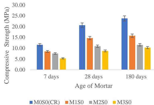
**Figure 9.** Effects of SDPMF content on mortars' compressive strength.
