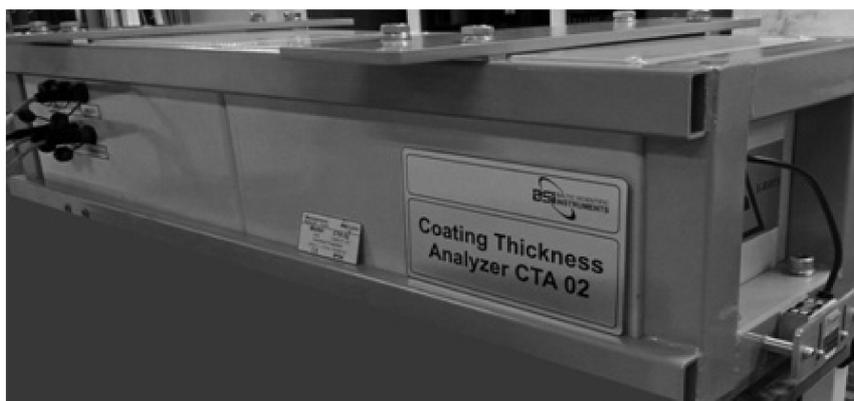
**Figure 2.** XRF gauge CTA-02 analyzer with optoelectronic displacement sensor (at the bottom of the frame on the right).
