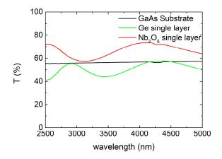
**Figure 5.** Optical transmittance spectra of the GaAs substrate, the Ge single layer and the Nb<sub>2</sub>O<sub>5</sub> single layer.
