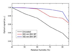
**Figure 10.** Measured optical signal as a function of increasing RH for uncoated, 160 nm BW BP, and 300 nm BW BP-coated sensors. It can be seen that the uncoated sensor was the most sensitive to increasing  $H_2O$  concentration, due to the sharp drop-off of the optical signal vs RH curve, therefore successfully demonstrating that by application of the narrow BPF, sensitivity to  $H_2O$  vapour is reduced.
