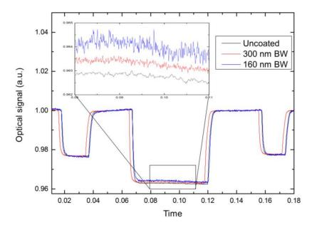
**Figure 9.** Calibrated sensor signal response for uncoated, 160 nm BW bandpass (BP)-coated and 300 nm BW BP-coated sensors when cycled from 0, 25,000, and 50,000 ppm methane (LEL) over the course of 4 h. The inset plot shows an exploded view of the signal at 5% methane, highlighting the different noise characteristic between the uncoated, 300 nm BW BP-coated sensor and the 160 nm BW BP-coated sensor.
