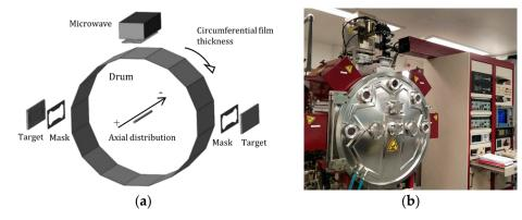
**Figure 4.** (a) Schematic of the microwave plasma-assisted sputter reactor used to deposit the thin optical films described in this work, and (b) the image of the actual chamber. Right- and left-hand-side magnetrons were used, populated with Ge on Nb target material.
