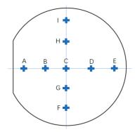
**Figure 11.** Schematic of a 4" Si wafer as mounted onto the microwave plasma-assisted sputter coater drum. Post-coating, the wafer was diced into  $20 \times 20 \text{ mm}^2$  sections, and the optical transmittances were measured for samples A–I to test for coating thickness uniformity. This was assessed for both the 300 nm and 160 nm BW bandpass filters.
