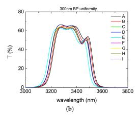
**Figure 12.** (a) Optical transmittance spectral characteristics for different Si wafer location samples A–I for the 160 nm BW bandpass filter; (b) Optical transmittance spectral characteristics for different Si wafer location samples A–I for the 300 nm BW bandpass filter.
