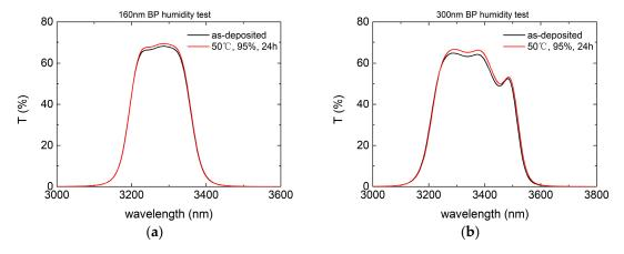
**Figure 14.** Optical transmittance of (a) the 160 nm and (b) the 300 nm BW bandpass witness sample after a humidity test.
