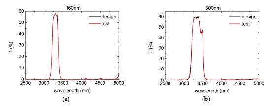
**Figure 7.** Comparison between theory and experiment for (a) the 160 nm BW bandpass filter and (b) the 300 nm BW bandpass filter designs.
