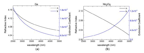
**Figure 6.** Optical constants for (a) thin film Ge and (b) thin film Nb<sub>2</sub>O<sub>5</sub> as calculated by using a combination of the O'Leary, Johnson and Lim (OJL) and Drude models.
