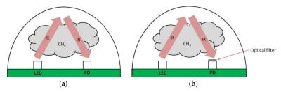
Figure 1. Schematic of the CH<sub>4</sub> gas sensor (a) without and (b) with an optical filter.
