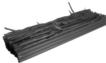
**Figure 8.** Tubular plastic wood model after a serrated tool was drawn across its surface.
