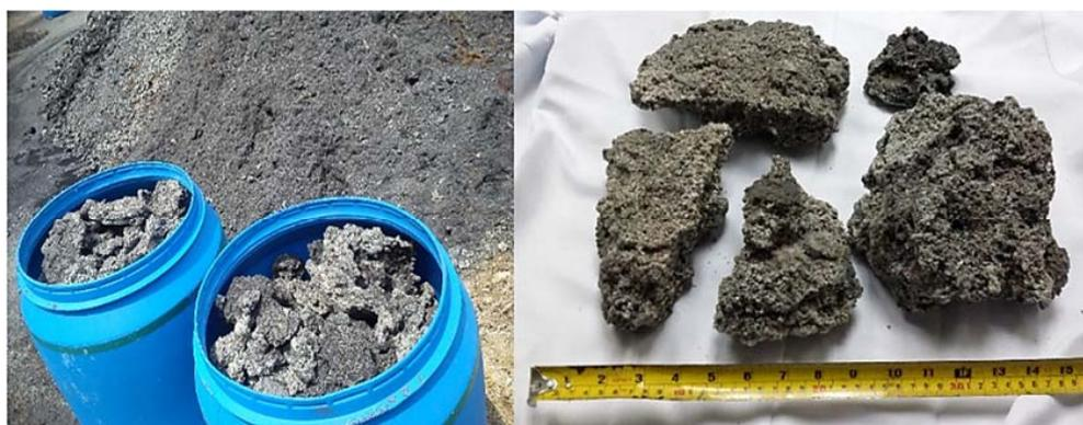
Figure 2. Raw POC collected from palm oil mill.
