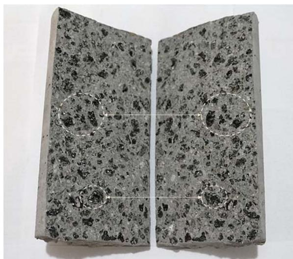
Figure 16. Splitting tensile failure.
