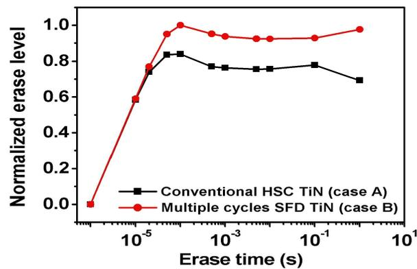
Figure 10. Normalized erase level change of devices for conventional FDC and GETiN gates.
