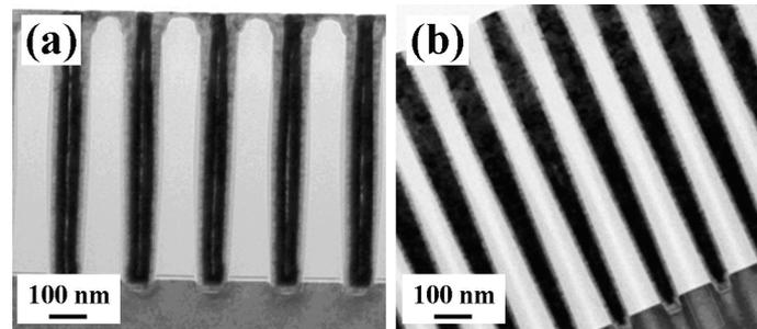
**Figure 7.** TEM images of fill-in performance on special funnel-like profile. (a) MOCVD TiN; (b) High aspect ratio of 12:1 deep contact with SFD TiN barrier.
