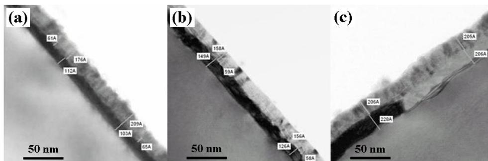
**Figure 2.** Cross-sectional TEM images of PECVD  $\text{TiCl}_4$ -based Ti covered with same TiN films at (a) 550 °C; (b) 600 °C; (c) 650 °C.
