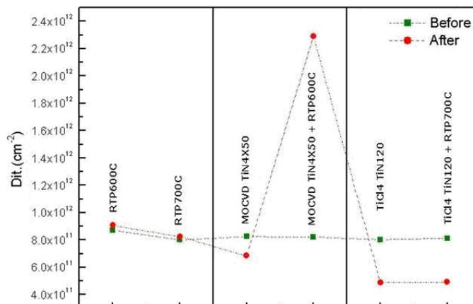
**Figure 5.** MOCVD TiN's impurity is activated by RTP thermal which shows much higher  $D_{it}$  than that of  $\text{TiCl}_4$ -based TiN.
