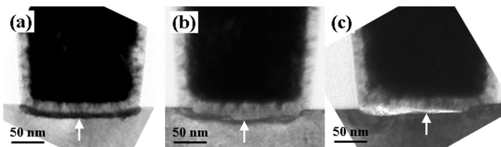
**Figure 3.** Contact bottom profiles for  $\text{TiSi}_x$  formation at (a) 550 °C; (b) 600 °C; (c) 650 °C. The arrowhead represents the  $\text{TiSi}_x$  formation quality.
