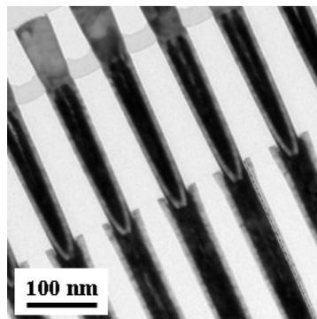
**Figure 8.** TEM image of plug performance in advanced small via application based on CVD  $\text{TiCl}_4$ -based TiN.
