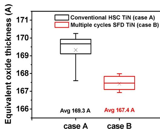
**Figure 9.** Distribution characteristic of equivalent oxide thickness in devices with different TiN gates.
