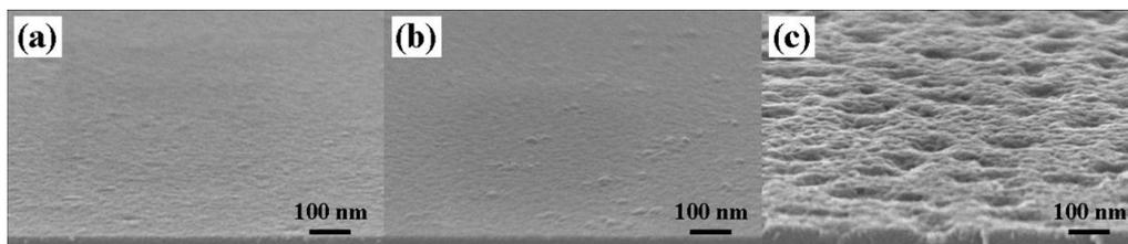
**Figure 1.** SEM images of PECVD  $\text{TiCl}_4$ -based Ti films on Si surface at process temperatures of (a) 550 °C; (b) 600 °C; (c) 650 °C.
