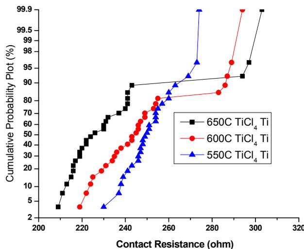
**Figure 4.** Cumulative probability plot of contact resistance for PECVD  $\text{TiCl}_4$ -based Ti at different process temperatures.
