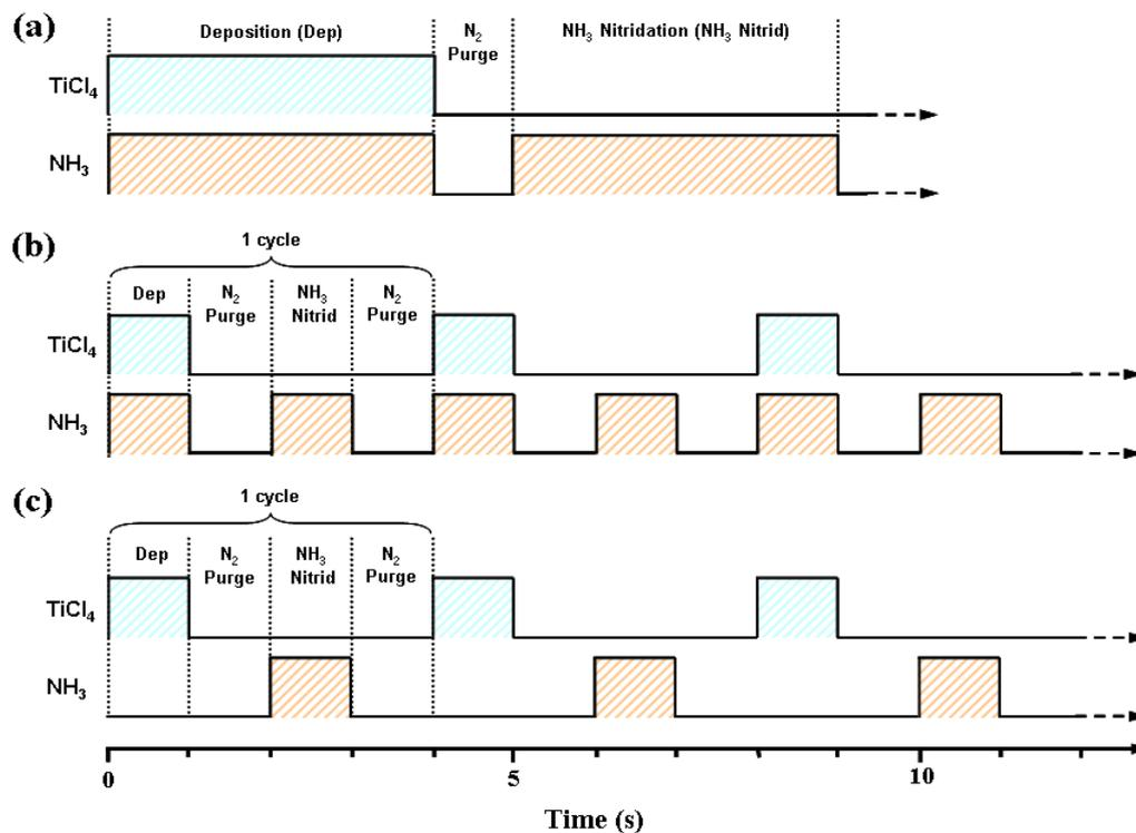
**Figure 6.** Schematic diagrams of the precursor flow steps of (a) conventional HSC; (b) SFD; (c) ALD TiN deposition methodologies.
