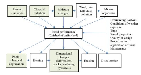
Figure 1. Elements in the weathering process.
