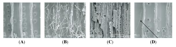
**Figure 7.** Scanning electron microscope of brown-rot fungal attack on wood. (**A**) control; (**B**,**C**) 51.1% weight loss after the 12 weeks in the ASTM soil block test; (**D**) acetylated pine after the soil block test.
