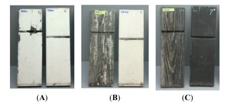
Figure 10. Photographic impression performance of opaque white (A,B) and black (C) coatings after 9<sup>1</sup>/<sub>2</sub> years of outdoor exposure. (A) opaque white acrylic, left control, right acetylated; (B) opaque white alkyd, left control, right acetylated; (C) opaque black alkyd, left control, right acetylated. [16].
