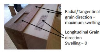
**Figure 5.** Stile and rail door part showing swelling of the control (left) and no swelling in the acetylated door (right). No longitudinal swelling in either control or acetylated wood but radial and tangential swelling in the control but not in the acetylated wood.
