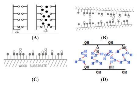
**Figure 2.** Models of water added to the wood cell wall. (A) Water molecules entering the wood cell wall; (B) water molecules unzipping hydrophylic polymer chains; (C) water bonding to the cell wall either as primary water  $\bullet$  or secondary water  $\circ$ ; (D) fully hydrated cell wall at the fiber saturation point.
