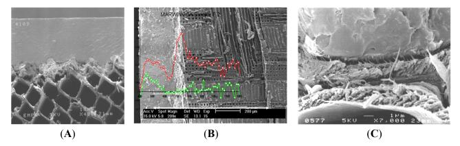
Figure 4. Coating on the surface of the wood (A); moisture gradient at the interface of the coating and the wood (B); and coating delamination (C).
