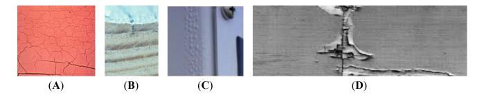
**Figure 3.** Cracking of surface coating due to differential swelling of the coating and wood (**A**); micro checks occur in the wood due to moisture evasion and swelling (**B**); water collecting under coated wood (**C**); and coating failure due to moisture build up in end grain (**D**).
