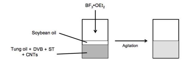
**Figure S1.** Sample preparation for the cationic polymerization of tung oil-based thermosetting resins.
