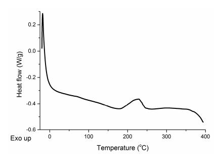
**Figure S2.** DSC curve of a tung oil-based resin reinforced with 0.25 wt % CNTs microwaved at 100 W for 10 min, followed by 200 W for 10 min, and a 1 h 30 min post-cure step at 140 °C in a convection oven.
