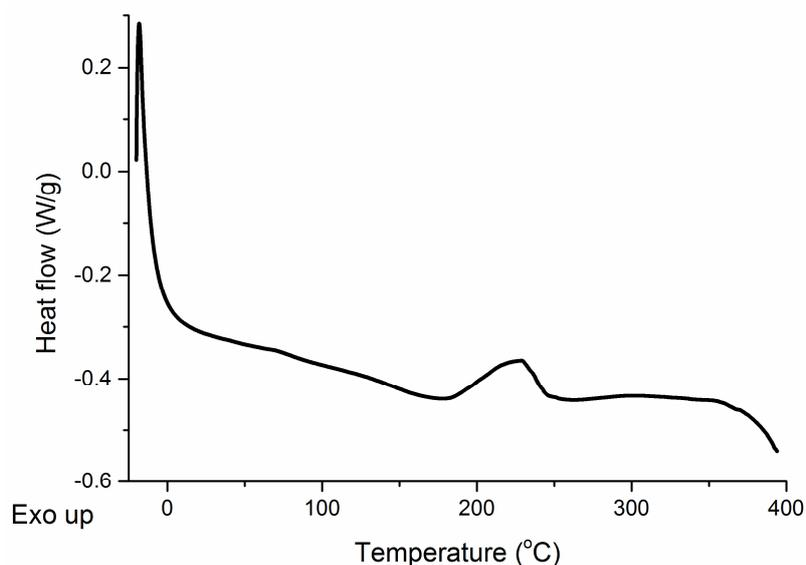
**Figure S2.** DSC curve of a tung oil-based resin reinforced with 0.25 wt % CNTs microwaved at 100 W for 10 min, followed by 200 W for 10 min, and a 1 h 30 min post-cure step at 140 °C in a convection oven.
