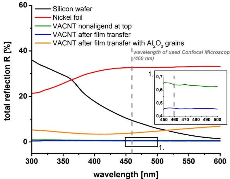
**Figure S1.** Spectra of total reflexion measurements of the substrates, grown VACNT at nickel foil, and VACNT at primer-coated aluminum foil after film transfer.
