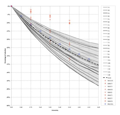
**Table 9.** Overall thermal transmittance of the wall built with the evaluated block: percentage of reduction.
