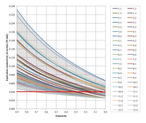
Values of thermal resistance of the evaluated block are shown in Table 4. A reduction in the equivalent thermal conductivity of the enclosures produces an increase in the thermal resistance value of the block of +32%–82% (Table 5), from values of 2.65–0.96 m<sup>2</sup>·K/W ( $\epsilon = 0.9$ ) to values of 4.20–1.34 m<sup>2</sup>·K/W ( $\epsilon = 0.1$ ) (Table 4).
