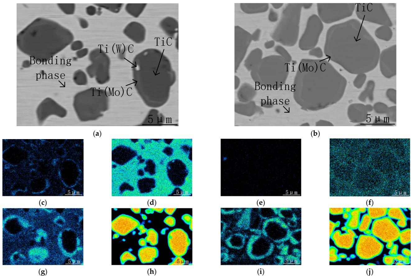
**Figure 2.** Element distribution in PMZ. (a) Multi-alloy strengthened microstructure; (b) non-strengthened microstructure; (c) W distribution in (a); (d) Cr distribution in (a); (e) W distribution in (b); (f) Cr distribution in (b); (g) Mo distribution in (a); (h) Ti distribution in (a); (i) Mo distribution in (b); (j) Ti distribution in (b).
