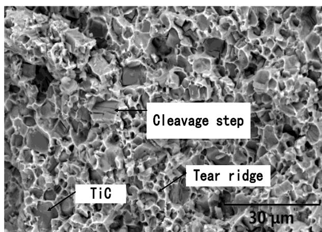
**Figure 4.** Optimal composition of arc-welded TiC cermet interface fracture.
