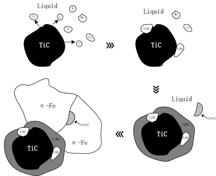
**Figure 5.** Microstructure evolution of TiC cermet arc welding.
