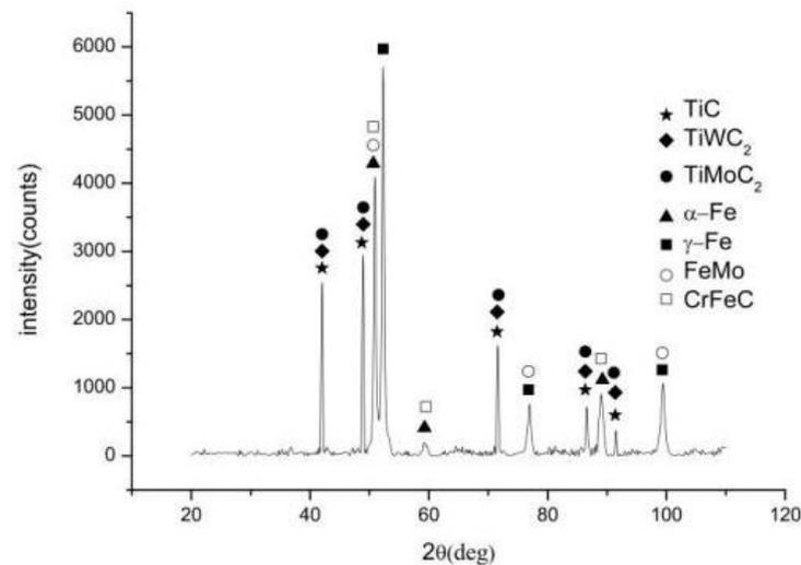
**Figure 3.** XRD test of the welded interface.
