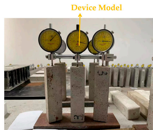
Figure 5. The testing process of DSR for SAA-RPC.
