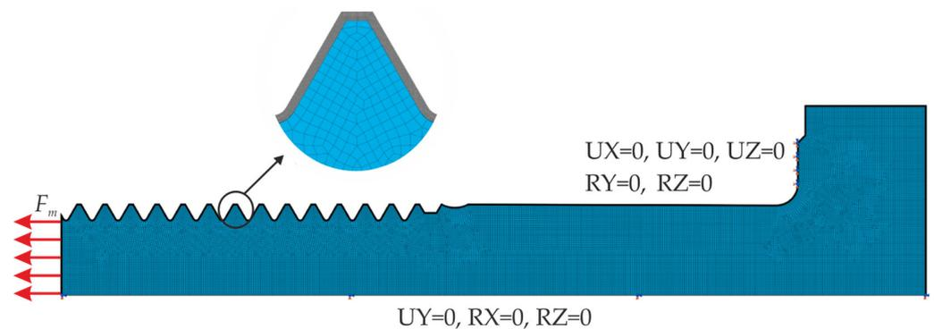
**Figure 2.** Example of a zinc-coated bolt FE model.**Table 4.** Characteristics of the FE mesh for the zinc-coated models.
