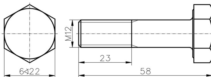
**Figure 1.** Dimensions of the tested bolts.
