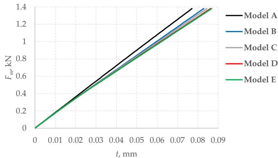
**Figure 3.** Force–displacement diagrams for the adopted bolt models.
