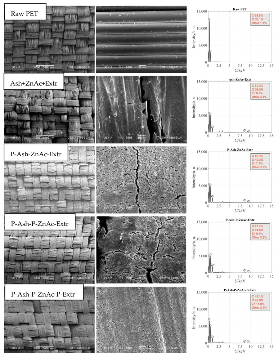
**Figure 3.** SEM micrographs and EDS analysis of raw PET and samples "Ash+ZnAc+Extr", "P-Ash-ZnAc-Extr", "P-Ash-P-ZnAc-Extr", and "P-Ash-P-ZnAc-P-Extr".
