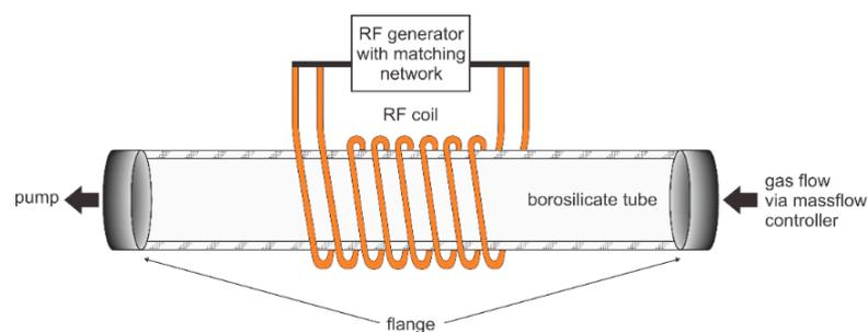
**Figure 2.** Schematic presentation of plasma system used.
