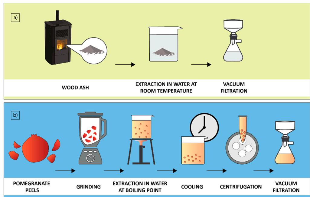
**Figure 1.** Schematic presentation of wood ash extract (a) and pomegranate peel extract (b) preparation.
