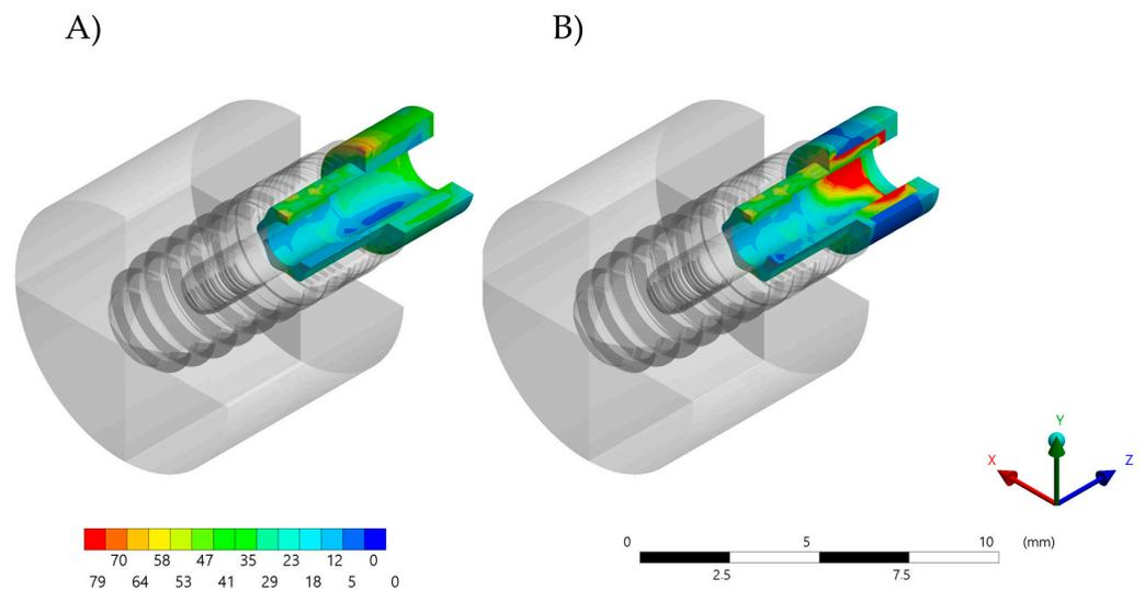
**Figure 8.** Von-Mises stress maps (MPa) in the abutment. (A) Zirconia abutment and (B) Bio-HPP abutment.
