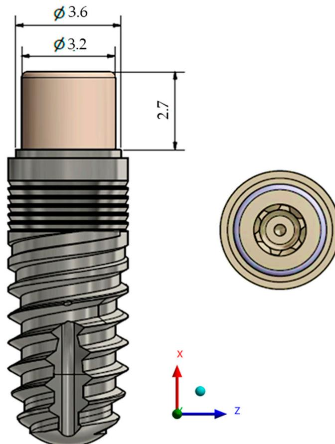
**Figure 1.** Schematic illustration of the experimental abutment design in lateral and occlusal views.
