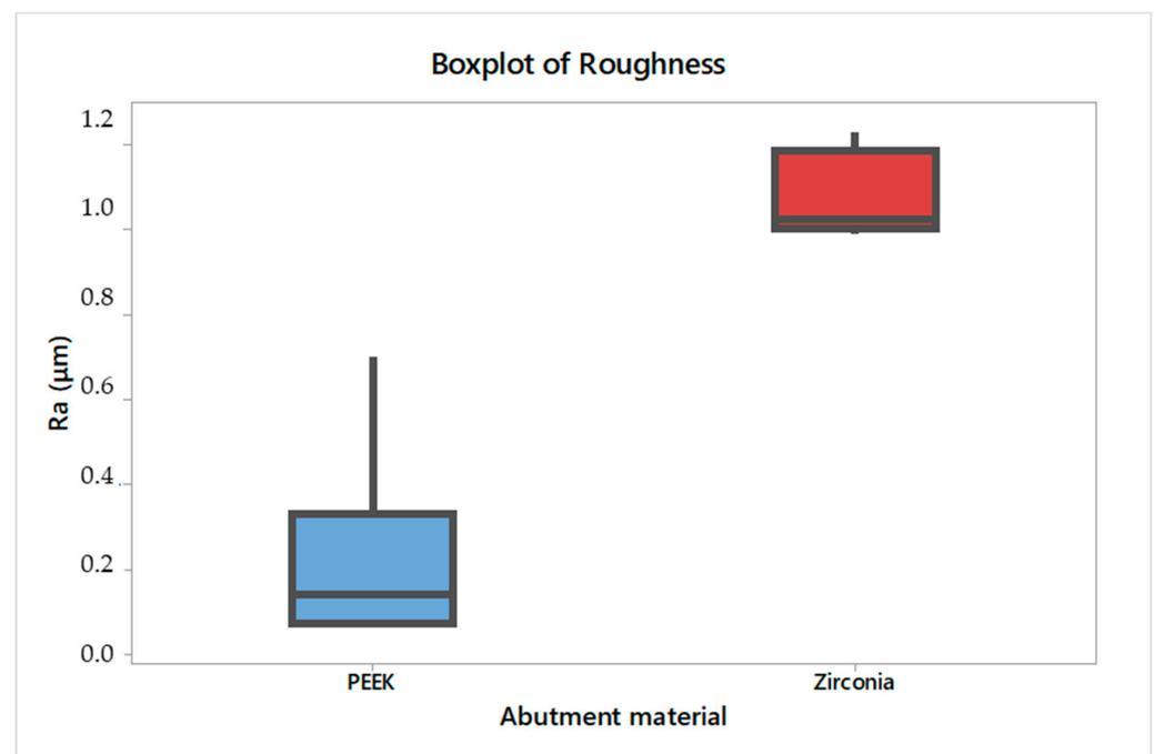
**Figure 3.** Boxplot of average roughness (Ra) according to the abutment material.
