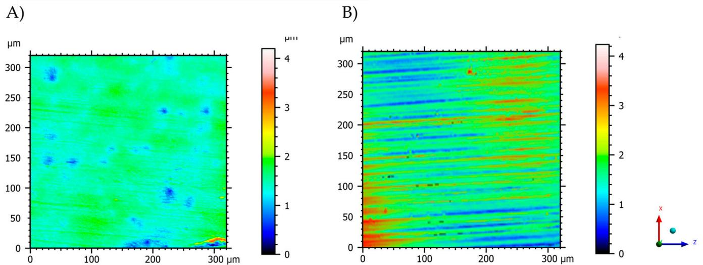
**Figure 4.** Representative images of the surface topography with shaped removed, showing different topographic patterns. (A) Bio-HPP and (B) Zirconia abutment.
