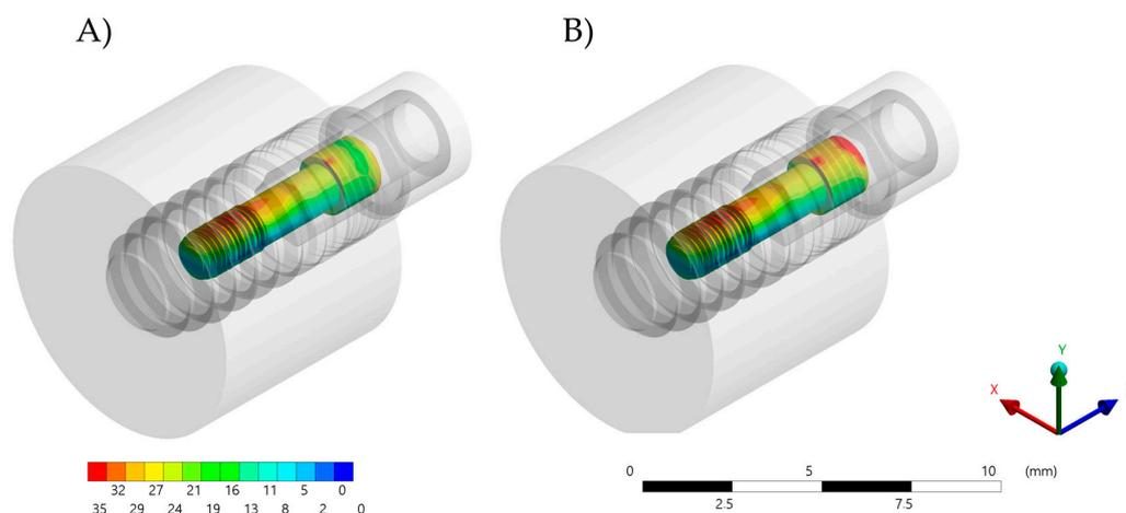
**Figure 9.** Von-Mises stress maps (MPa) in the screw. (A) Zirconia abutment and (B) Bio-HPP abutment.
