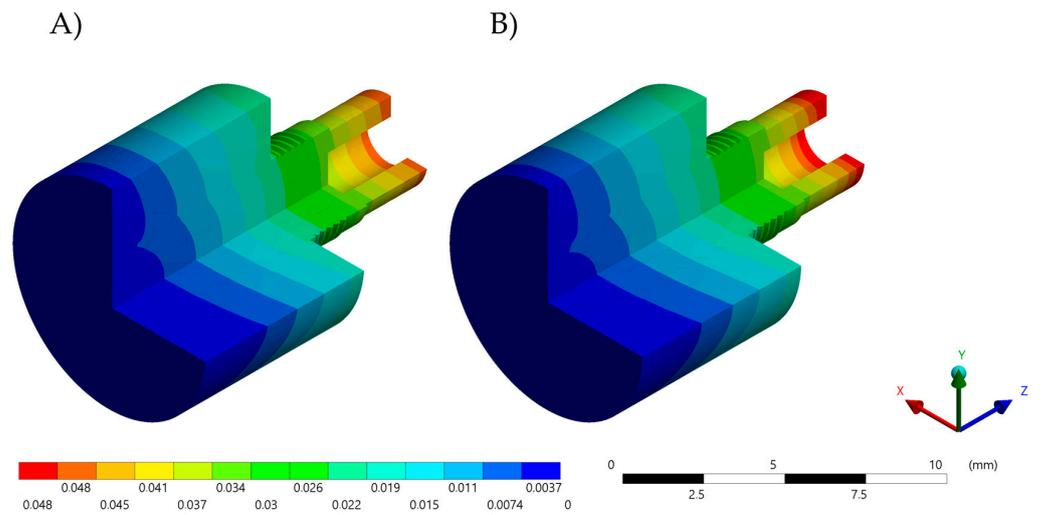
**Figure 6.** Convergence results verification using Total Deformation (mm). (A) Zirconia abutment and (B) Bio-HPP abutment.
