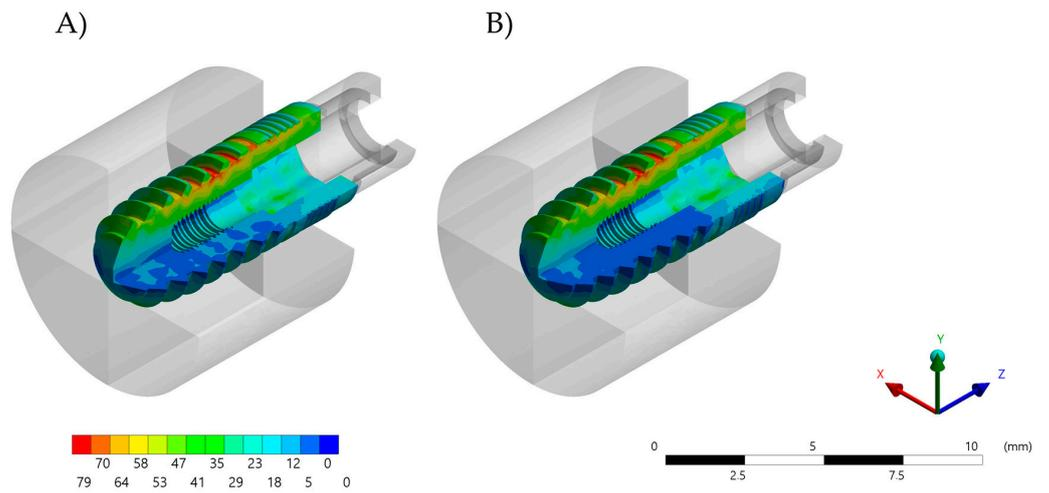
**Figure 7.** Von-Mises stress maps (MPa) in the implant fixture. (A) Zirconia abutment and (B) Bio-HPP abutment.
