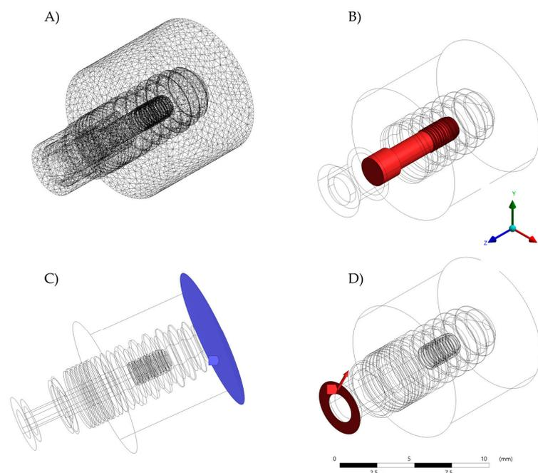
**Figure 2.** Numerical model and boundary conditions. (A) Mesh model containing implant, (B) bolt pre-tension, (C) Fixed support at the base and (D) Force load applied on the top.
