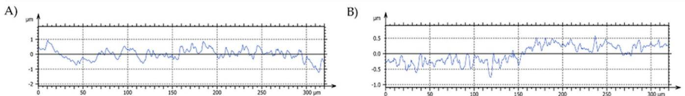
**Figure 5.** Representative profile cut (vertical) including waviness for Zirconia (A,B) Bio-HPP samples.
