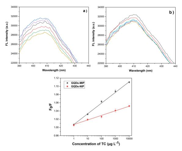
**Figure 5.** Fluorescence emission spectra of GQDs-MIPs (**a**) and GQDs-NIPs (**b**) with the addition of various amounts of TC in water.  $F_0$  and F represent the fluorescent intensities before and after the addition of TC solution, respectively.
