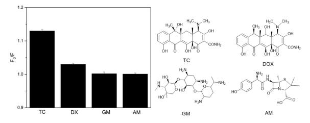
**Figure 6.** Selective adsorption of TC, DOX, GM and AM by GQDs-MIPs in water. The concentration of all compounds was  $10^4 \ \mu g \ L^{-1}$ .
