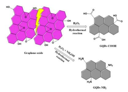
Figure 1. Illustration of the preparation of GQDs from graphene oxide.
