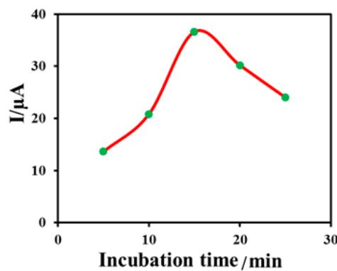
**Figure S1.** The effect of the enzyme incubation time on the current responses of the modified electrode.
