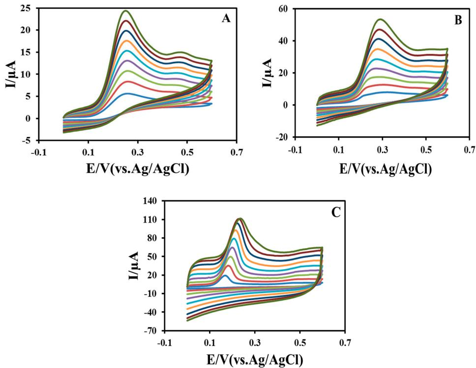
**Figure S2.** Cyclic Voltammograms of INZ with (A) Bare GCE, (B) MWCNT-GCE, (C) MWCNT-TiO<sub>2</sub>NP-GCE at various scan rates: 0.1, 0.2, 0.3, 0.4, 0.5, 0.6, 0.7, 0.8 and 0.9 V·s<sup>-1</sup>.
