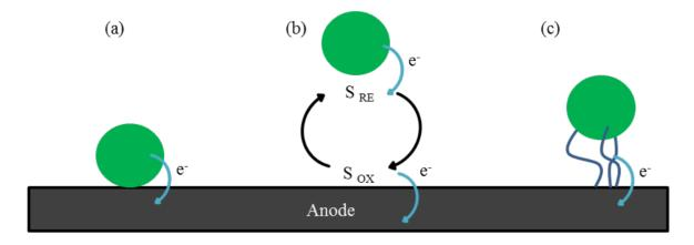
**Figure 2.** A schematic of three electron transfer mechanisms of microbes at the anode surface: (a) direct transfer by contact; (b) indirect electron transfer by redox shuttles (S  $_{RE}$  = reduced electron shuttle, S  $_{OX}$  = oxidized electron shuttle); (c) electron transfer by conductive nanowire matrix.
