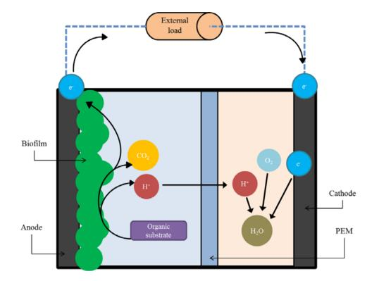
**Figure 1.** Operating principles of a two-chamber microbial fuel cell (not to scale). The electroactive biofilm at the anode break down an organic substrate to produce electrons, protons and  $CO_2$ . The electrons pass through an external load to be reduced at the cathode.
