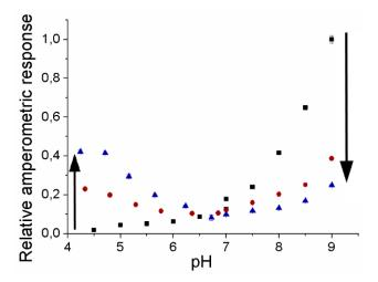
The addition of KCl results in a decrease of the response of the PaoABC-biosensor in the alkaline region and increase of response in acidic solutions from no response up to 40% of the highest amperometric response at pH 9, while the response around pH 6.5 is low and not influenced (Figure 3).
