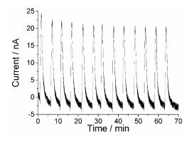
The sensor response is repeatable (Figure 7) with 1.9% relative standard deviation in a series (n = 13, 200  $\mu$ M benzaldehyde). The variation between three sensors is 14% for the measurement of 200  $\mu$ M benzaldehyde. Sixty-eight percent of the initial sensitivity was retained after five days of measurements, when the sensor was stored refrigerated between the daily measurements.
