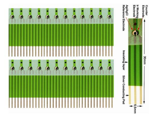
**Figure 2.** Screen-printed single-use, disposable Ir nano-catalyst contained  $H_2O_2$  platform biosensor prototype.
