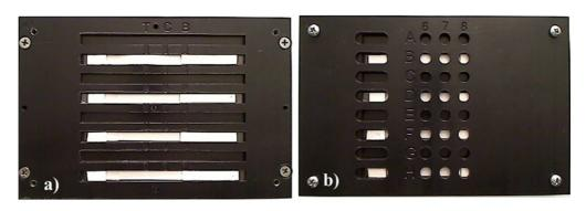
Up to eight test strips could be read at one time using the holder device. For the microtiter plate reader, the chemiluminescent intensity was quantified over time. The chemiluminescent/time curve was then integrated. CCD imaging was used for assay optimization and to generate images. Data are reported as averages  $\pm$  standard deviation of at least n=3 replicates. Results are representative of at least three independent experimental trials.
