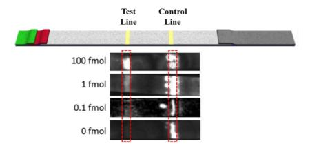
**Figure 4.** Chemiluminescence at both the test lines and controls lines were quantified using a microtiter plate reader over 60 min. At low target amounts such as this (0.1 fmol), the control line appears much stronger than the test line.
