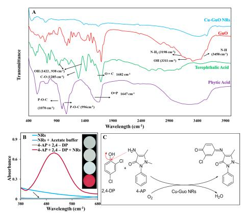
**Figure 2.** (**A**) FTIR spectra of phytic acid, terephthalic acid, Guo, and Cu-Guo NRs. (**B**) The absorbance spectra of NRs, the mixture of NRs and acetate buffer, and 2,4-DP and 4-AP in the absence and presence of NRs nanozyme with their corresponding images, and (**C**) a proposed reaction mechanism of 2,4-DP and 4-AP catalyzed by Cu-Guo NRs nanozyme.
