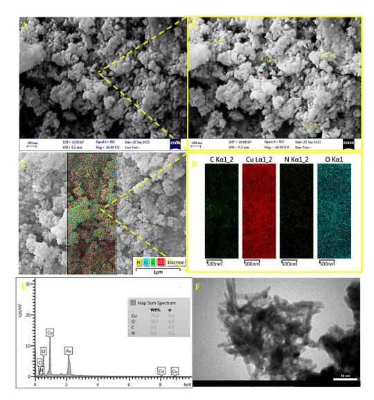
**Figure 1.** (**A**,**B**) SEM images, (**C**–**E**) EDX analysis and elemental mapping, and (**F**) TEM image of the synthesized Cu-Guo NRs.
