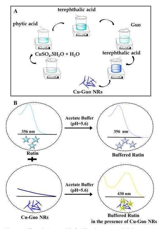
**Scheme 1.** (**A**) The synthesis process of Cu-Guo NRs as the nanozyme and (**B**) the sensing strategy of the proposed sensor using Cu-Guo NRs for Rtn measurement.
