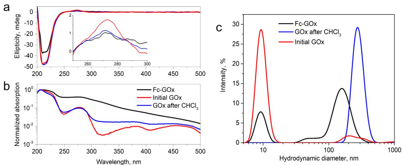
**Figure 1.** Spectroscopic characterization of Fc-GOx: (a) CD spectra of the Fc-GOx, unaffected (initial) GOx and GOx after its exposure in  $\text{CHCl}_3$  samples ( $c = 1 \text{ mg mL}^{-1}$ ) and (b) UV–Vis ( $c = 0.25 \text{ mg mL}^{-1}$ ); (c) the measured hydrodynamic diameters of Fc-GOx, initial GOx, and GOx after its exposure in  $\text{CHCl}_3$  ( $c = 1 \text{ mg mL}^{-1}$ ). All the samples were dissolved in the PPB pH 7.0 solution.
