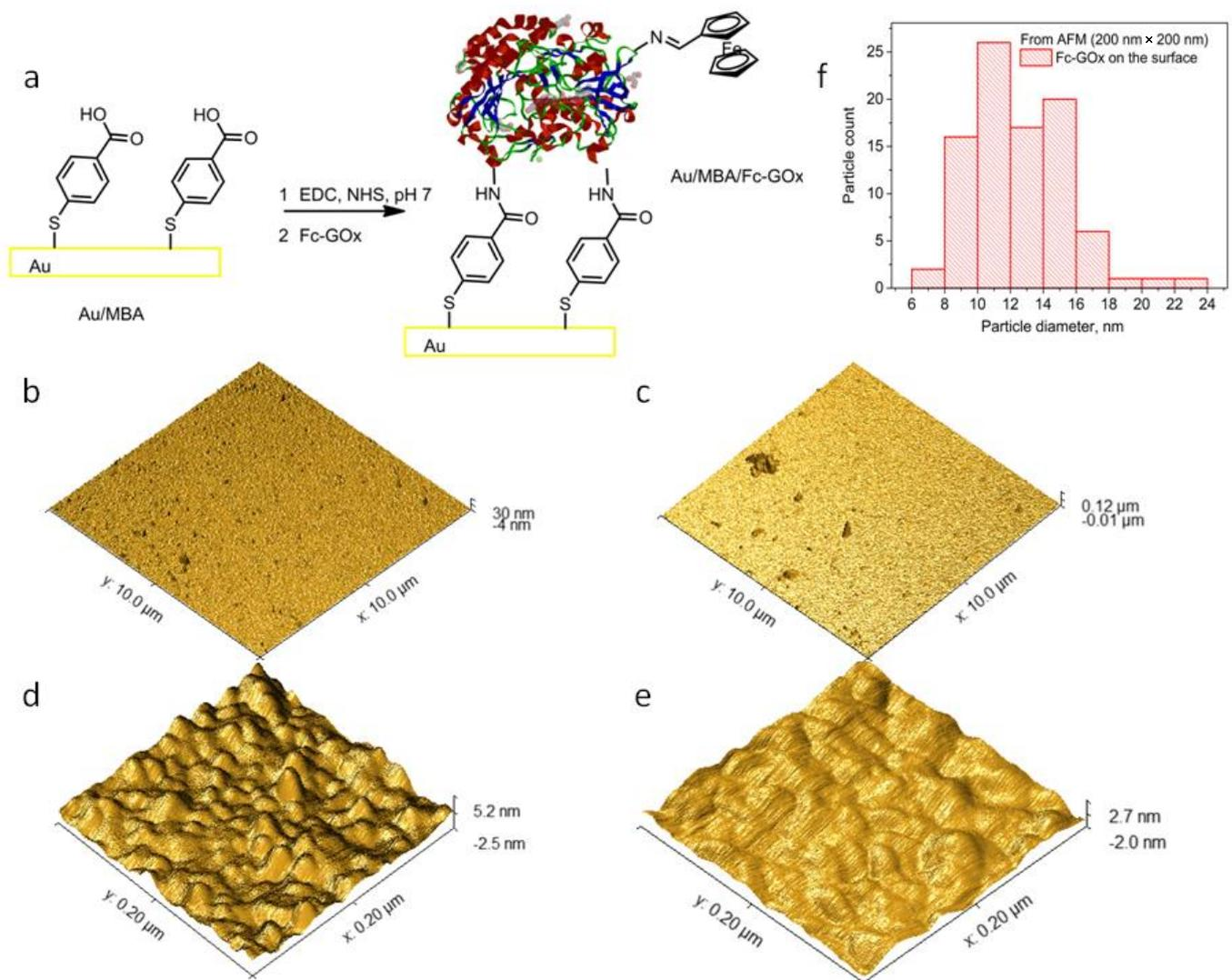
**Figure 2.** AFM analysis of the modified gold substrates: (a) schematic presentation of the self-assembly monolayer of Fc-GOx deposition on Au; (b) AFM picture of GOx/MBA/Au at dimensions of 10 × 10 μm; (c) AFM picture of Fc-GOx/MBA/Au at dimensions of 10 × 10 μm; (d) AFM picture of Fc-GOx/MBA/Au at dimensions of 200 × 200 nm; (e) AFM picture of the surface of bare Au at dimensions of 200 × 200 nm; (f) grain diameters distributions on the Fc-GOx/MBA/Au surface at dimensions of 200 × 200 nm.
