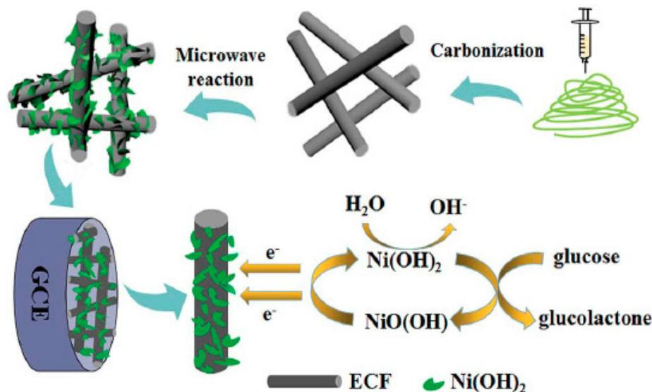
**Figure 4.** Ni(OH)<sub>2</sub>/ECNF nanocomposite fabrication steps. Reprinted from reference [106], with permission from the Royal Society of Chemistry.
