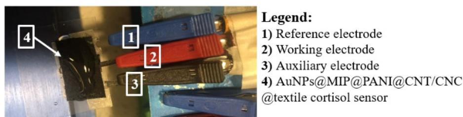
**Figure 1.** Camera image of the AuNPs@MIP@PANI@CNT/CNC@textile cortisol sensor patch and electrode orientation.
