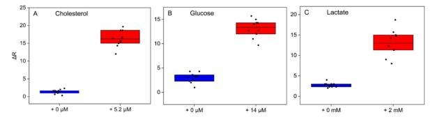
**Figure 2.**  $\Delta R$  values of the detection zones collected at the end of the assay (10 min) performed on native saliva (blue bars) and saliva spiked with (**A**) 5.2  $\mu$ M cholesterol, (**B**) 14  $\mu$ M glucose and (**C**) 2 mM lactate (red bars). Graphs provide the average result of 10 assays performed on saliva collected from 10 different donors.
