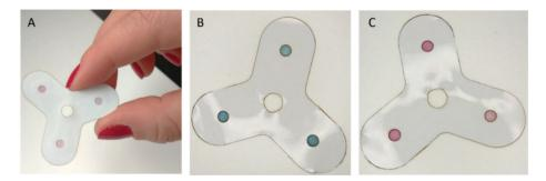
**Figure 7.** (**A**) Photograph of the final device embedded in the PVC mask with, representative of its real size. (**B**,**C**) Images of the proposed prototype with the specific mask after the assay on saliva spiked with the three analytes at the beginning of the test (**B**) and after 10 min of reaction (**C**).
