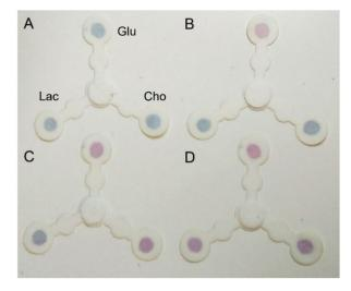
**Figure 5.** Photographs of four devices at the end of the reaction (10 min) treated respectively with (**A**) native saliva, (**B**) saliva spiked with one target biomarker (14  $\mu$ M glucose (Glu)), (**C**) saliva spiked with two targets (14  $\mu$ M glucose + 5.2  $\mu$ M cholesterol (Cho)), and (**D**) saliva spiked with all the targets (14  $\mu$ M glucose + 5.2  $\mu$ M cholesterol + 2 mM lactate (Lac)).
