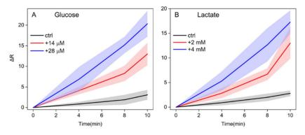
**Figure 3.**  $\Delta R$  values evolution over time of the detection zones after the assays on native saliva (black line), saliva spiked with the lowest (red line) and the highest (blue line) established non-physiological concentrations of (**A**) glucose (respectively, +14 and +28  $\mu$ M) and (**B**) lactate (respectively, +2 and +4 mM). The colored bands represent the standard deviation of 10 measurements performed on different salivary samples.
