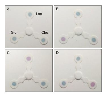
**Figure 4.** Representative photographs of the multiplexed devices after 10 min of reaction, treated with (**A**) native saliva, (**B**) saliva spiked with glucose (Glu) (14  $\mu$ M), (**C**) saliva spiked with lactate (Lac) (2 mM) and (**D**) saliva spiked with cholesterol (Cho) (5.2  $\mu$ M).
