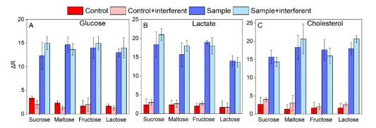
Figure 6.  $\Delta R$  values collected at the end of the assay (10 min) performed on native saliva (red histograms), saliva with interferents (pink histograms), saliva spiked with (A) 14  $\mu$ M glucose, (B) 2 mM lactate, and (C) 5.2  $\mu$ M cholesterol (dark blue histograms), and saliva spiked with a mix of the analytes and the interferents (light blue histograms). Error bars represents the uncertainty from three independent measurements.
