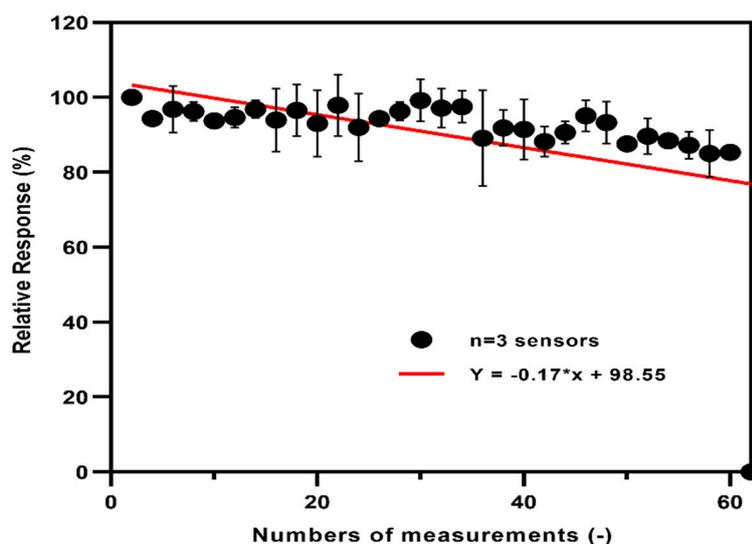
**Figure S4.** Operational stability of the GA sensor over 30 repeated measurements in 1 mM glucose solution in phosphate buffer. The graph depicts the average values of three individual sensors (mean  $\pm$  standard deviation); the red linear fit indicates the loss in measured current over the 30 cycles (total of 6 hours of measurement). The average remaining activity of the TEMPO-CNC glucose sensor after 30 measurements was 85.3 % of the initial current.
