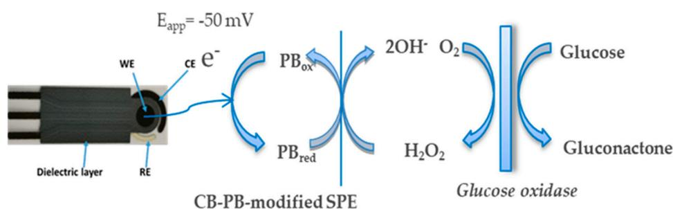
**Figure S1.** Schematic view of the sensor working principle. WE: working electrode, RE: reference electrode, CE: counter electrode.
