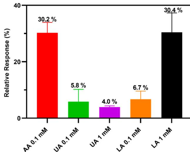
**Figure S3.** Relative responses of the GA sensor toward interfering species (0.1 mM ascorbic acid, 0.1 and 1 mM uric acid, 0.1 and 1 mM LA) in a 1 mM glucose standard solution in phosphate buffer. n = 3 for each condition; 1 mM glucose without interfering species is defined as 100 % response.
