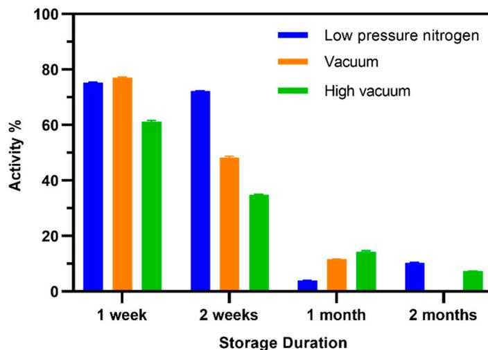
**Figure S5.** Shelf-life test of the GA sensor under different storage conditions: low-pressure nitrogen (400 mbar N<sub>2</sub>), vacuum ( $\leq 50$  mbar), and high-vacuum ( $\leq 10$  mbar) drying treatment before vacuum packing. All sensors were stored at 4 °C. The sensors were tested after 1 week, 2 weeks, 1 month, and 2 months. All values are normalized against the signals of sensors tested without storage.
