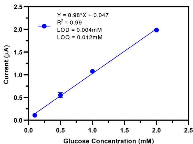
**Figure S2.** Calibration curve of the glutaraldehyde-based glucose sensor (GA sensor) in 0.1–2 mM glucose in phosphate buffer. The linear range (up to 2 mM) was smaller than the entire dynamic range. n = 3; plotted are the mean ± standard deviation and the linear fit from 0.1 to 2 mM.
