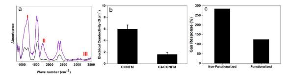
**Figure 5.** (a) ATR-FTIR showing the surface chemistry of  $a-CO_x/G$  nanofilaments as non-functionalized (black line) versus citric acid (CA)-functionalized (blue line) (I, II, and III represent C-O-C, C=O, and OH groups, respectively); (b) electrical conductivity of the carbon nanofilament-based membrane (buckypaper) as non-functionalized versus CA-functionalized; (c) toluene gas response of the  $a-CO_x/G$  buckypapers as CA-functionalized and non-functionalized.
