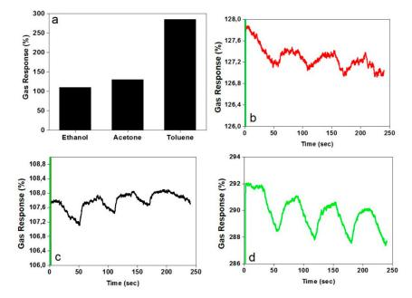
**Figure 4.** (a) Volatile organic compound (VOC) gas response of the a-CO<sub>x</sub>/G buckypapers; (b–d) the recovery property of the a-CO<sub>x</sub>/G buckypapers exposed to ethanol, acetone, and toluene, respectively.
