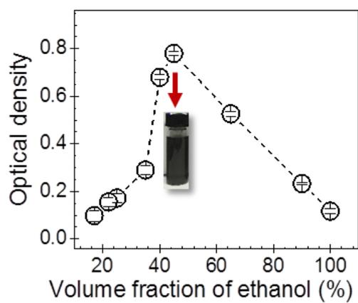
**Figure S1.** The optical densities of GNs dispersions obtained by exfoliating graphite in a series ethanol–water mixtures. It was found that the highest concentration of GNs dispersions was obtained in 45 vol% ethanol–water mixture. Therefore, in the study, the GNs were produced by exfoliating graphite in 45 vol% ethanol–water mixture.
