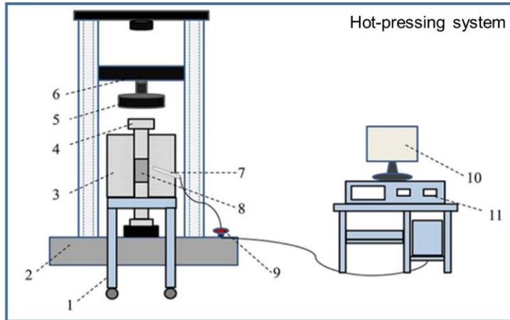
1 Base, 2 Electronic testing machine, 3 Heating furnace, 4 Pressure bar, 5 Indenter 6 Sensor, 7 Thermocouple, 8 Composite sample, 9 Switch, 10 Pressure control system 11 Temperature control system
