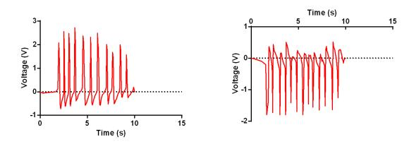
Figure S2. Voltage output in standard (left) and inverted (right) poles configuration.
