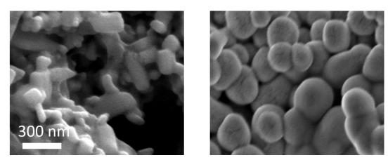
**Figure S1.** Dual Beam imaging of zinc oxide nanopowder (left) and barium titanate nanoparticles (right).
