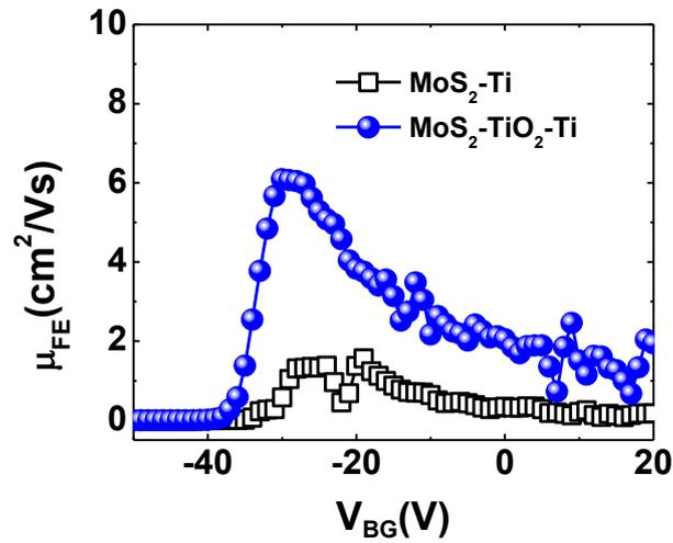
Figure S3. Field-effect mobility ( $\mu_{FE}$ ) for MoS<sub>2</sub> FETs without and with a TiO<sub>2</sub> layer.
