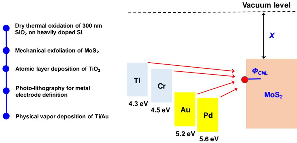
Figure S1. Fabrication process and band diagram for Fermi-level pinning with various metals.
