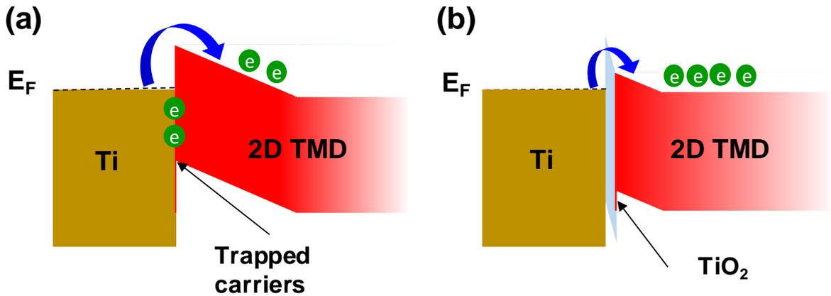
Figure S5. Energy band diagrams for TMDC-Ti and TMDC-TiO<sub>2</sub>-Ti stacks.
