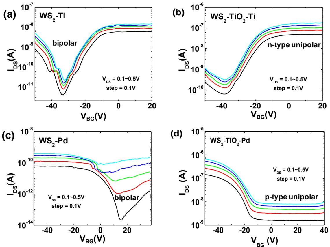
Figure S4. Transfer curves for WS<sub>2</sub>-Ti, WS<sub>2</sub>-TiO<sub>2</sub>-Ti, WS<sub>2</sub>-Pd, and WS<sub>2</sub>-TiO<sub>2</sub>-Pd structured FET devices.
