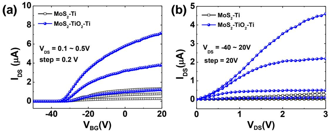
Figure S2. Transfer and output curves for MoS<sub>2</sub> FETs without and with a TiO<sub>2</sub> layer.
