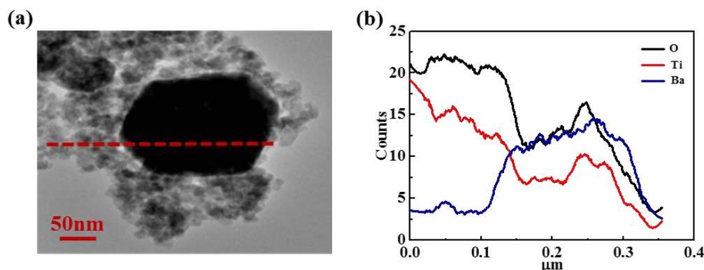
**Figure S4.** Line-scan EDS profile (b) along the red dot dash line crossing the BaTiO<sub>3</sub>-TiO<sub>2</sub> core-shell heterostructure (a).
