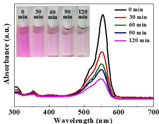
**Figure S5.** Absorption spectra of RhB solution in the presence of BaTiO<sub>3</sub>-TiO<sub>2</sub> core-shell heterostructures (1.2:1) under UV light irradiation. Inset shows color changes of the RhB solution.
