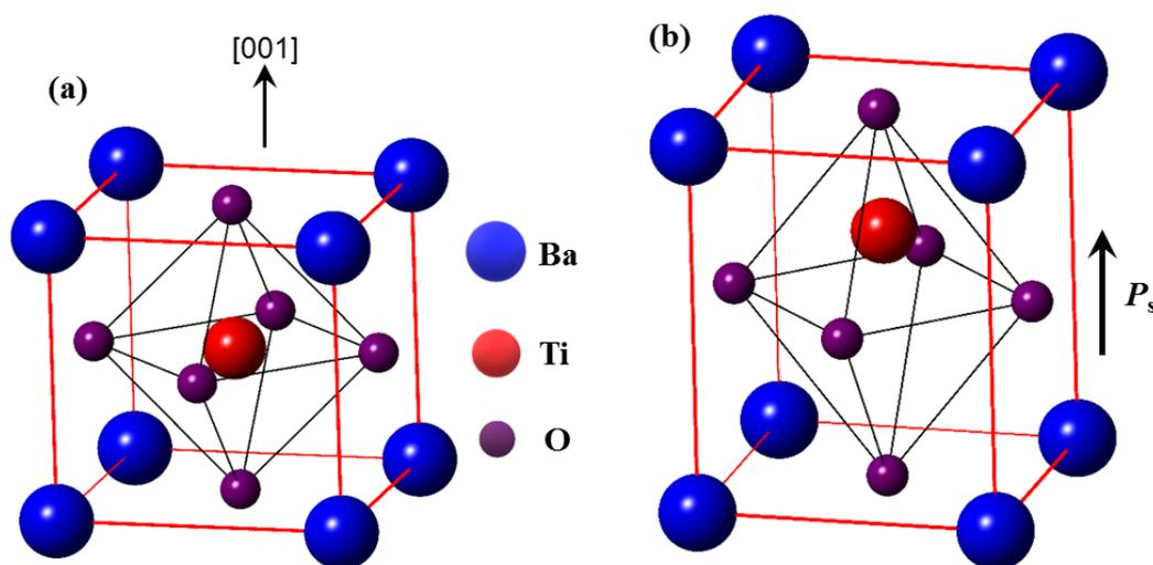
**Figure S1.** Crystal structure of (a) cubic (paraelectric) and (b) tetragonal (ferroelectric) BaTiO<sub>3</sub>.
