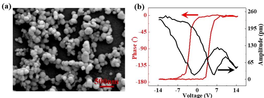
**Figure S2.** FESEM image (a) and (b) representative phase-voltage hysteresis loop (red) and amplitude-voltage butterfly loop (black) of BaTiO<sub>3</sub> after subjected to the hydrothermal process.
