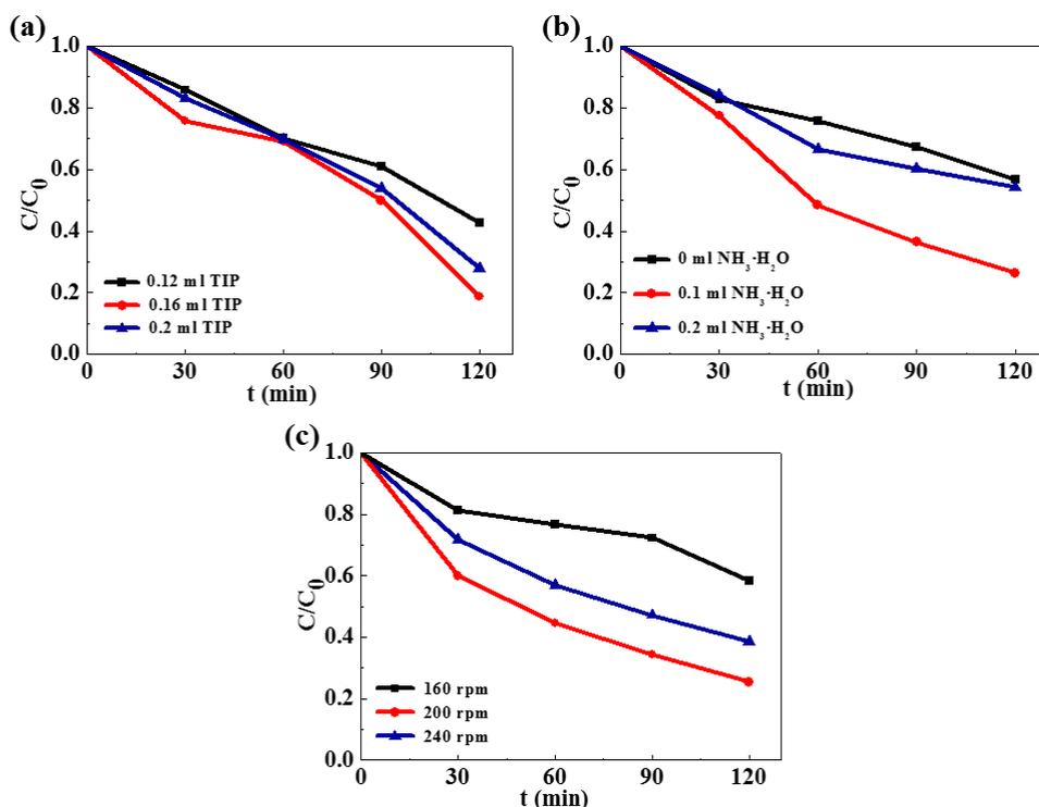
**Figure S3.** Photodegradation of RhB in the presence of catalysts synthesized at the different amount of TIP and NH<sub>3</sub>·H<sub>2</sub>O, and the varied stirring rate during the hydrolysis reaction.
