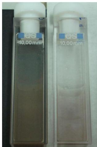
**Figure S3.** Photographs on dark and white backgrounds of quartz cells with a gold plating obtained from Au<sub>10</sub> clusters solution at acidic pH after 24 h.
