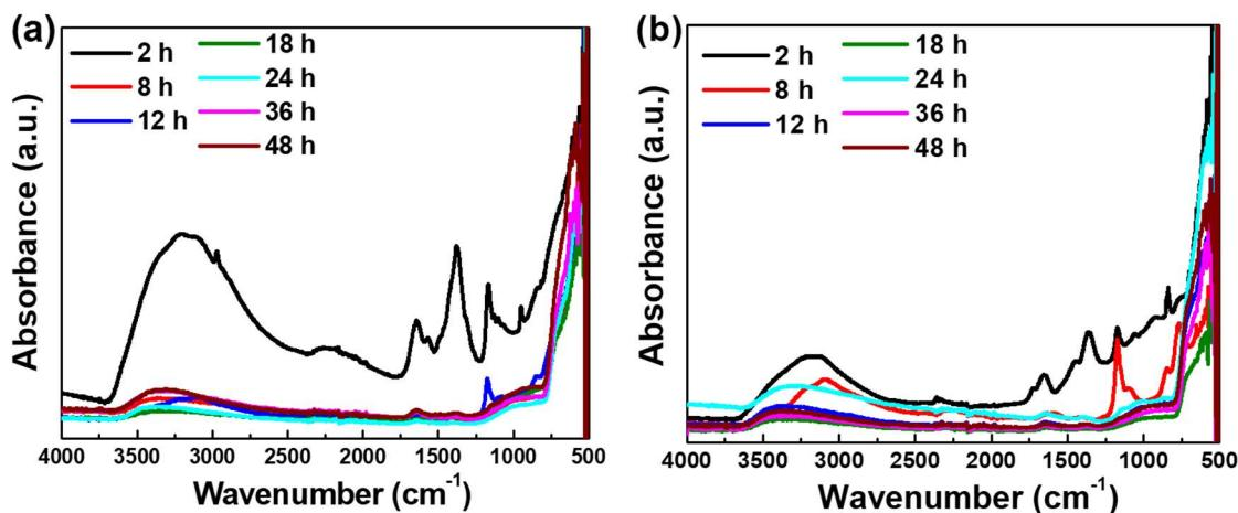
**Figure S10.** FTIR spectrum of samples with different reaction times for (a)  $\text{ZnCl}_2$  and (b)  $\text{ZnAc}$ .
