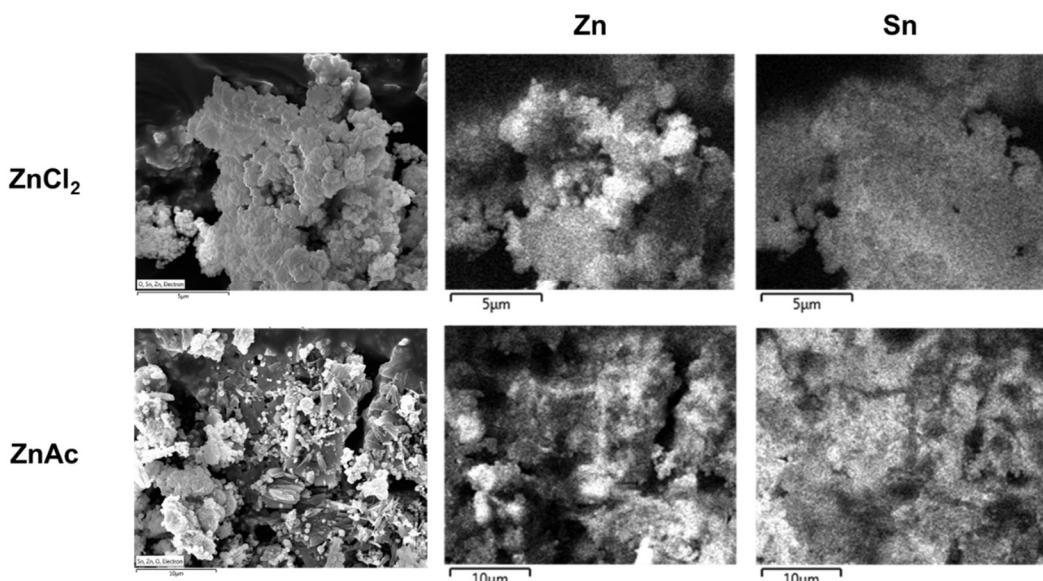
**Figure S11.** SEM image and EDS element mapping of nanostuctures produced by synthesis using (a)  $\text{ZnCl}_2$  (Zn:Sn molar ratio of 2:1) and (b)  $\text{ZnAc}$  (Zn:Sn molar ratio of 1:1), both at  $200\text{ }^\circ\text{C}$  for 2 h and a volume of 15 ml.
