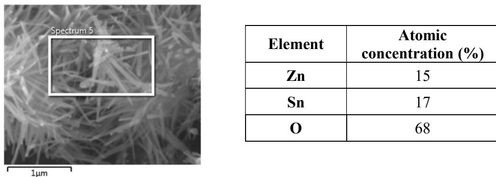
**Figure S2.** SEM image and EDS element quantification of ZnSnO<sub>3</sub> nanowires produced by synthesis using ZnCl<sub>2</sub>, a Zn:Sn molar ratio of 2:1, a volume 15 ml at 200 °C for 24 h. This analysis shows Zn:Sn ratio of 1:1, supporting identification of the ZnSnO<sub>3</sub> phase. The higher than expected atomic concentration of oxygen can be attributed to the carbon tape.
