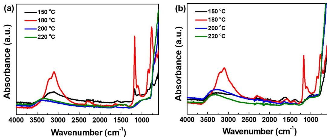
**Figure S5.** FTIR spectra of the obtained nanostructures using (a)  $\text{ZnCl}_2$  and (b)  $\text{ZnAc}$ , at different temperatures ( $150\text{ }^\circ\text{C}$ ,  $180\text{ }^\circ\text{C}$ ,  $200\text{ }^\circ\text{C}$  and  $220\text{ }^\circ\text{C}$ ).
