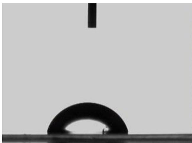
**Figure S2.** A water contact angle of  $72^\circ$  was obtained on the Ag/PET hybrid nanostructures.
