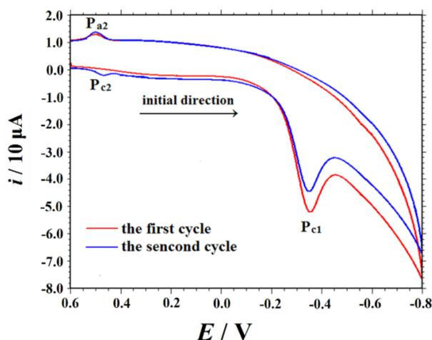
**Figure 3.** Cyclic voltammograms by continuous sweep cycles recorded on GR/ABPE (Concentration:  $10 \mu\text{M}$  4-NP in  $0.1 \text{ M HCl}$  solution, Scan rate:  $0.1 \text{ V s}^{-1}$ ).
