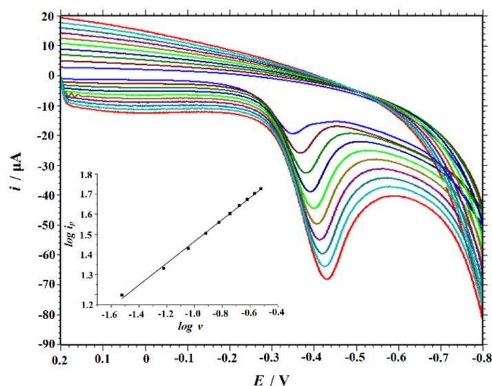
**Figure 4.** Cyclic voltammograms of GR/ABPE immersed in 10  $\mu\text{M}$  4-NP and 0.1 M HCl solution under different scan rates in the range  $0.03 \text{ V s}^{-1}$  to  $0.3 \text{ V s}^{-1}$ ; Inset: linear relationship fitting between  $\log i$  and  $\log v$ .
