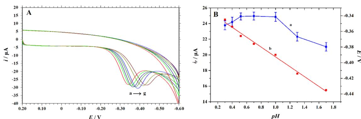
**Figure 7.** (A) Cyclic voltammograms recorded on GR/ABPE in  $10\ \mu\text{M}$  4-NP and  $0.1\ \text{M}$  HCl solution with different pH values (from a to g are 0.30, 0.40, 0.52, 0.70, 1.00, 1.30, 1.70, respectively, scan rate:  $0.1\ \text{V s}^{-1}$ ); (B) the peak current and pH relationship while error bars represent SD,  $n = 3$  (curve a); the linear relationship between the peak potential and pH (curve b).
