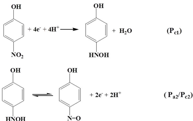
**Scheme 1.** The electrochemical reaction mechanism of 4-NP on the GR/ABPE.
