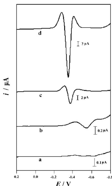
**Figure 6.** Second-order derivative linear sweep voltammograms recorded on (a) graphite powder (CPE), (b) ABPE, (c) GR/CPE and (d) GR/ABPE. (Concentration: 10  $\mu\text{M}$  4-NP and 0.1 M HCl, accumulation conditions: 0.0 V, 60 s, scan rate: 0.1  $\text{V s}^{-1}$ ).
