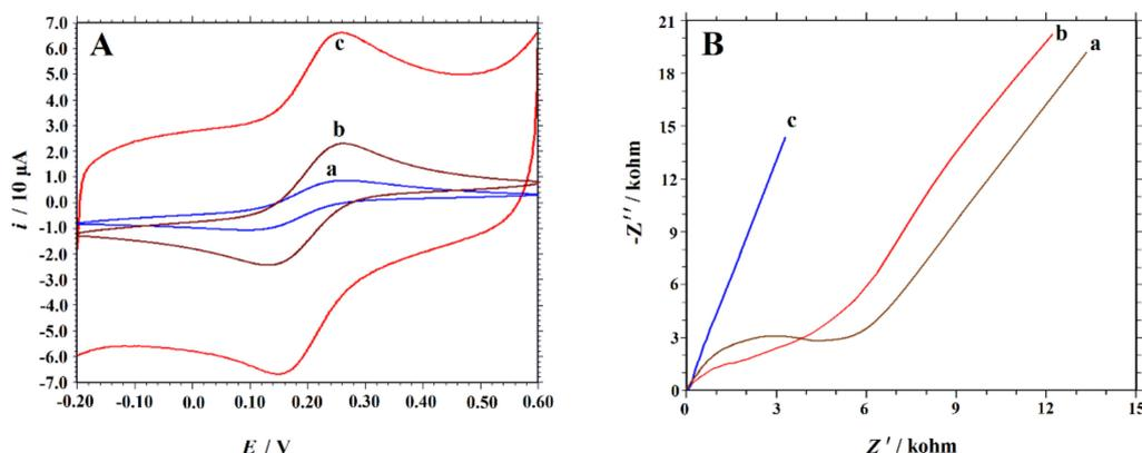
**Figure 1.** Cyclic voltammograms (A) and Nyquist plots (B) of different electrodes in 1.0 mM  $K_3[Fe(CN)_6]$  solution containing 0.5 M KCl. Scan rate:  $0.1 \text{ V s}^{-1}$ . The frequency range was from 0.1 to  $10^5$  Hz at the formal potential of 0.17 V. (a) CPE, (b) ABPE, (c) GR/ABPE.
