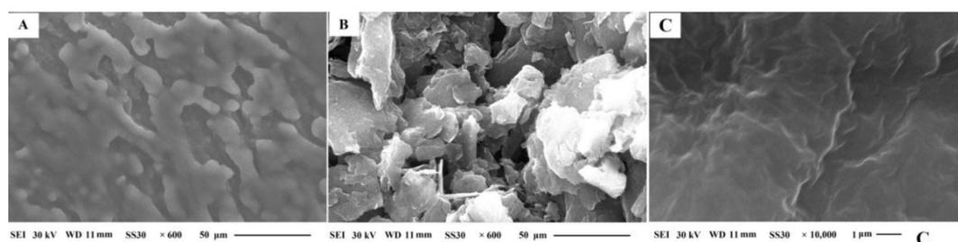
**Figure 2.** SEM images sampled from (A) acetylene black paste electrode (ABPE), (B) graphene and acetylene black paste hybridized electrode (GR/ABPE) at low magnification and (C) GR/ABPE at high magnification.
