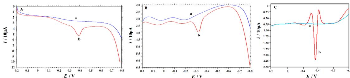
**Figure 5.** Linear sweep voltammetry (LSV) (A); differential pulse voltammetry (DPV) (B); and second-order derivative linear sweep voltammetry (C) of 0.1 M HCl (curve a) 0.1 M HCl containing 5.0  $\mu\text{M}$  4-NP (curve b) recorded on GR/ABPE after accumulated at 0.0 V for 60 s. Scan rate: 0.1  $\text{V s}^{-1}$ .
