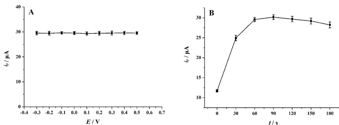
**Figure 8.** (A) Effect of accumulation potential and (B) accumulation time on the peak current of  $10\ \mu\text{M}$  4-NP in  $0.1\ \text{M}$  HCl solution on GR/ABPE, error bars represent SD,  $n = 3$ ; accumulation time was 60 s in Figure 8A.
