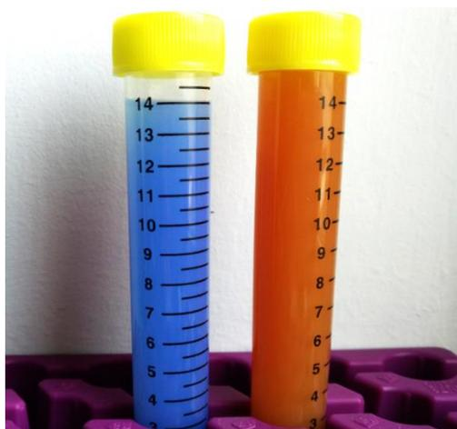
**Figure S2.** A photograph of Cu(OH)<sub>2</sub> nanocages colloid before (left) and after (right) introducing N<sub>2</sub>H<sub>4</sub>. Note that the color of hydrazine-treated solutions was the same at a stoichiometric N<sub>2</sub>H<sub>4</sub> amount and excess N<sub>2</sub>H<sub>4</sub> added to Cu(OH)<sub>2</sub> nanocages.
