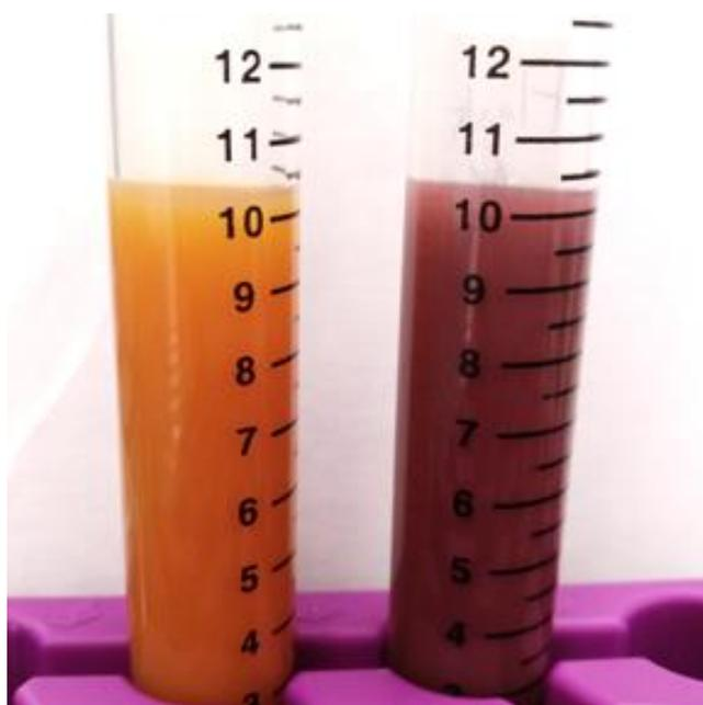
**Figure S4.** A photograph of  $\text{Cu}_2\text{O-N}_2\text{H}_4$  colloid (obtained by treating  $\text{Cu}(\text{OH})_2$  nanocages in ethanol with hydrazine ( $[\text{N}_2\text{H}_4]:[\text{Cu}(\text{OH})_2] = 5$ ) immediately after hydrazine addition (left) and after aging the mixture for 2 days (right).
