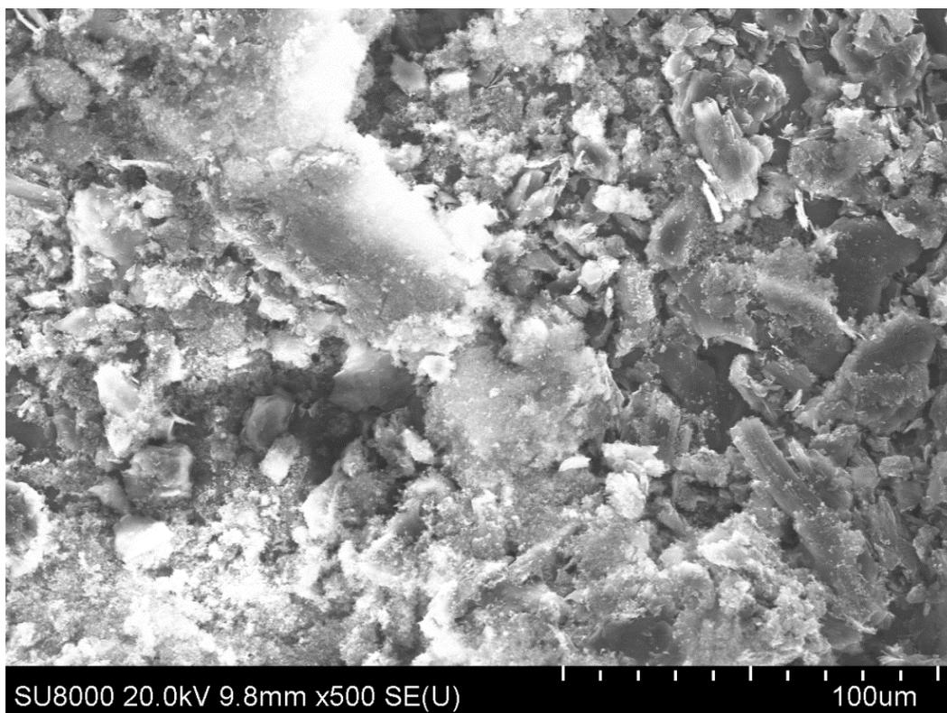
**Figure S199.** SEM image of graphite powder with  $ZrO_2-SiO_2$  sample after MW treatment.
