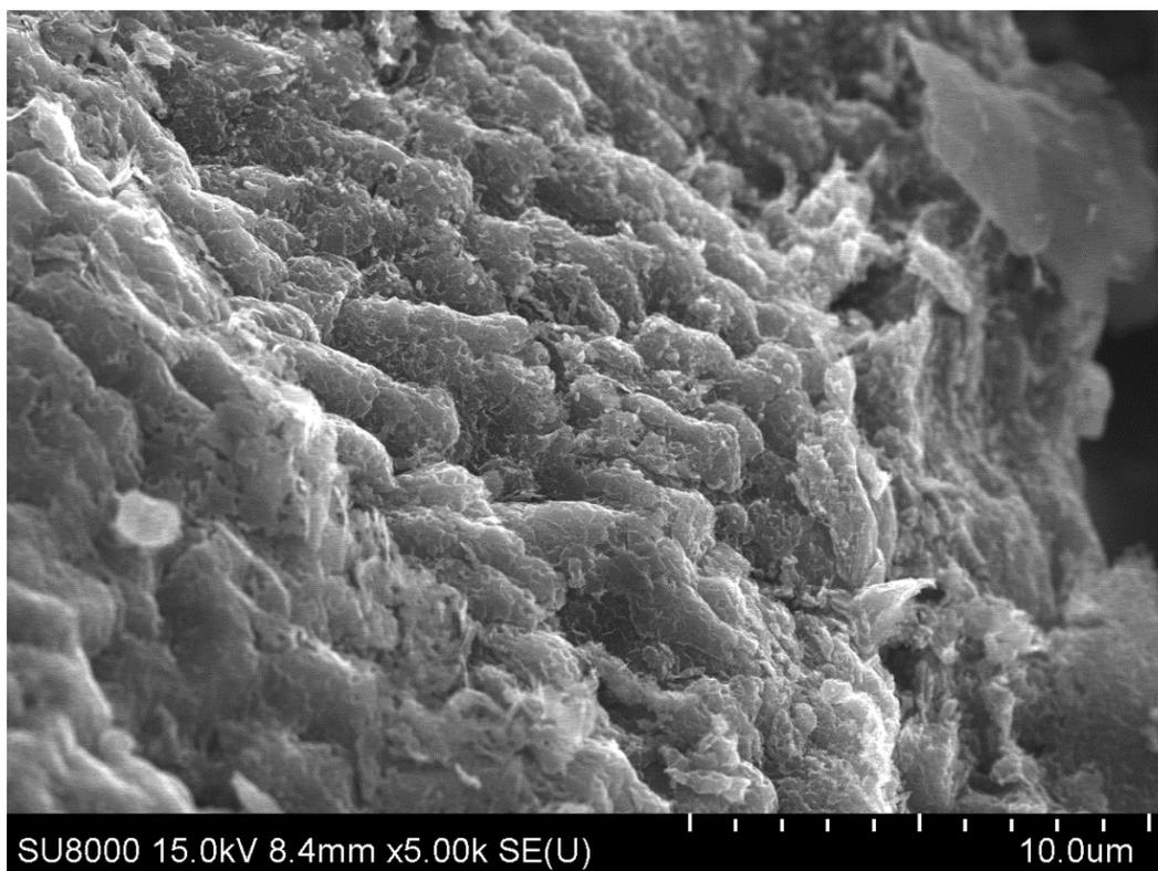
**Figure S129.** SEM image of graphite powder with Cu-W sample after MW treatment.
