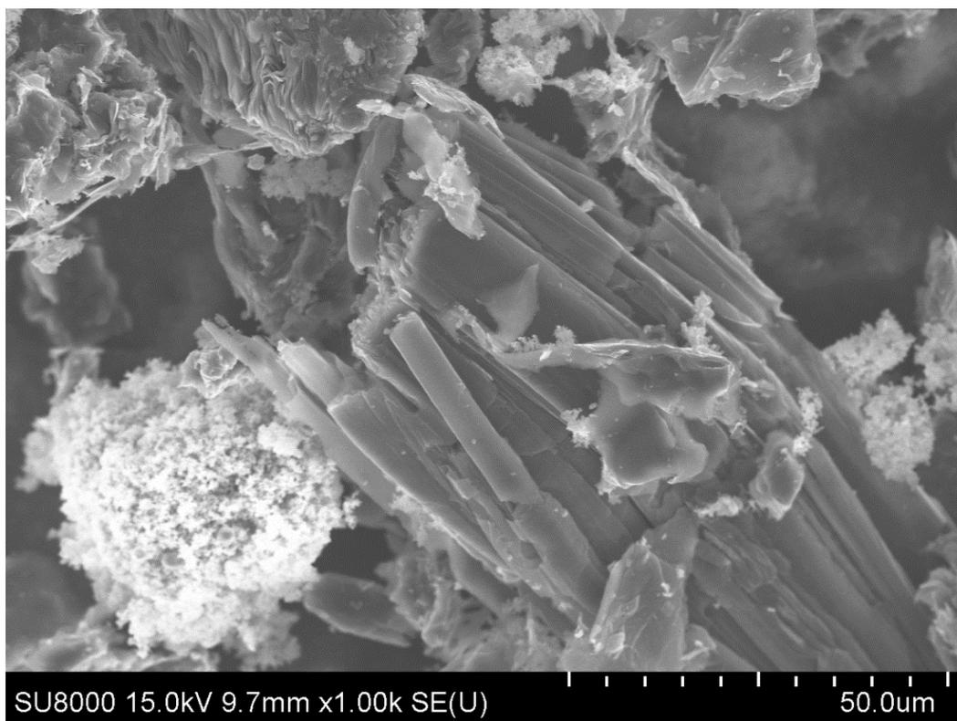
**Figure S142.** SEM image of graphite powder with TiCN sample after MW treatment.
