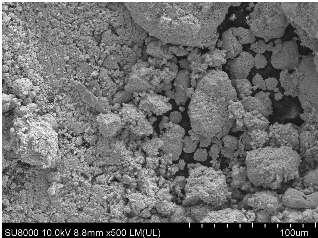
Figure S91. SEM image of initial sample of W-V-C powder.
