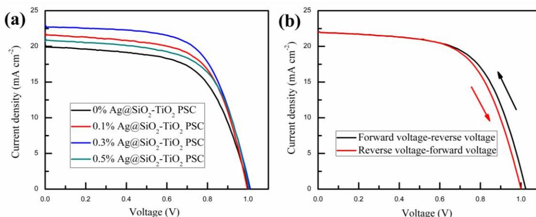
**Figure 6.** (a)  $J$ - $V$  curves of PSC devices based on mesoporous  $\text{TiO}_2$  film mixed with different amounts of  $\text{Ag@SiO}_2$  NPs; (b)  $J$ - $V$  curves scanned from forward voltage to reverse voltage and scanned from reverse voltage to forward voltage.
