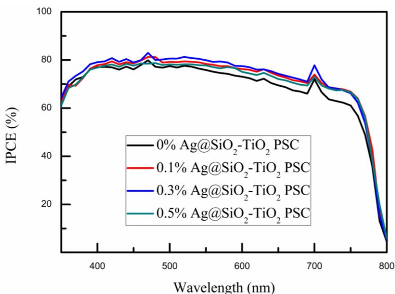
**Figure 8.** IPCE spectra of PSC devices based on mesoporous TiO<sub>2</sub> film mixed with different amounts of Ag@SiO<sub>2</sub> NPs.
