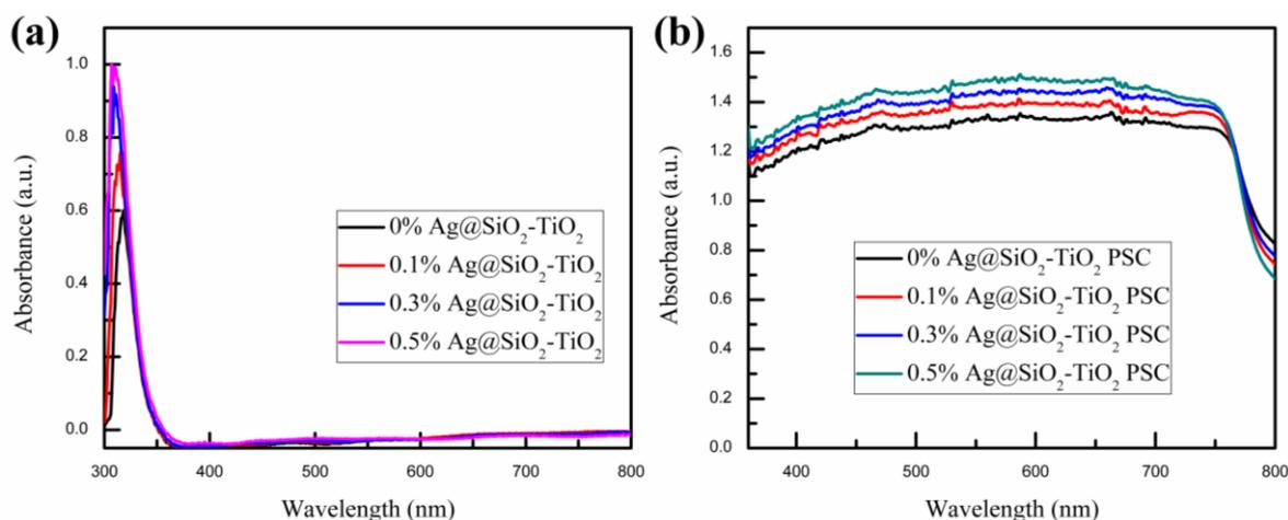
**Figure 5.** UV-vis absorption spectra of (a) pristine TiO<sub>2</sub> and TiO<sub>2</sub> mixed with Ag@SiO<sub>2</sub> NPs mesoporous film samples and (b) PSCs with pristine TiO<sub>2</sub> and TiO<sub>2</sub> mixed with Ag@SiO<sub>2</sub> NPs mesoporous film.
