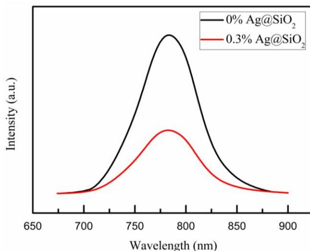
**Figure 9.** PL spectra of compact TiO<sub>2</sub>/Ag@SiO<sub>2</sub>-TiO<sub>2</sub>/ZrO<sub>2</sub>/perovskite films at room temperature of 296 K.
