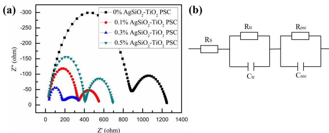
**Figure 10.** (a) Nyquist curves of the PSC devices based on different amounts of Ag@SiO<sub>2</sub> NPs films and (b) the equivalent circuit employed to fit the plots.
