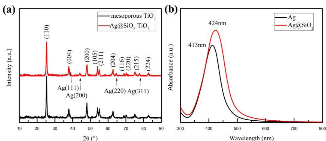
**Figure 2.** (a) XRD patterns of mesoporous TiO<sub>2</sub> and the Ag@SiO<sub>2</sub>-TiO<sub>2</sub>; (b) Optical absorption spectra of 26 nm-Ag NPs and Ag@SiO<sub>2</sub> NPs dispersed in alcohol.
