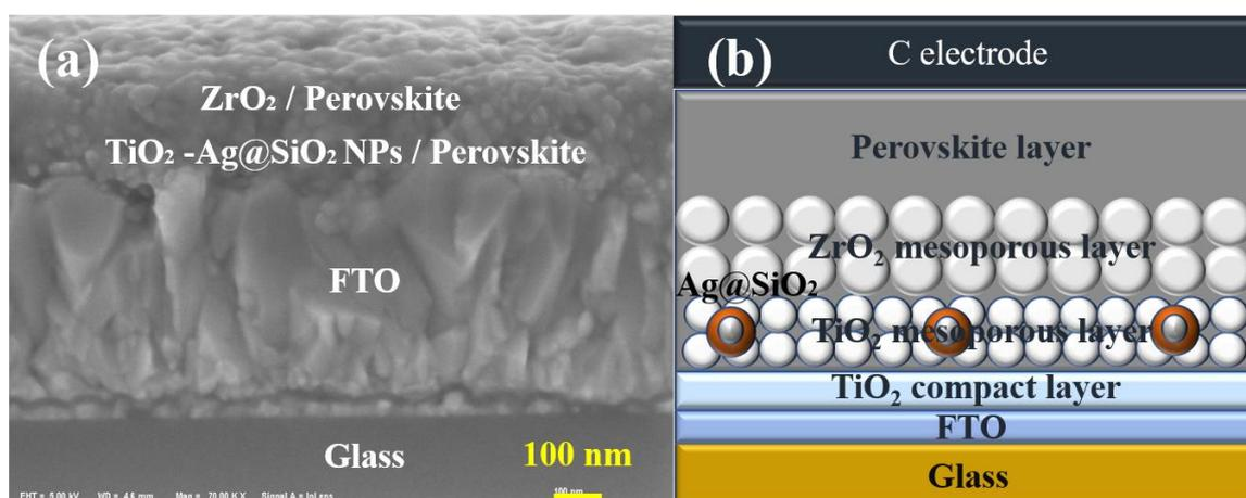
**Figure 4.** (a) Scanning Electron Microscope (SEM) image of a cross section of a complete PSC mixed with Ag@SiO<sub>2</sub> NPs; (b) Structural representation of a whole PSC device mixed with Ag@SiO<sub>2</sub> NPs.
