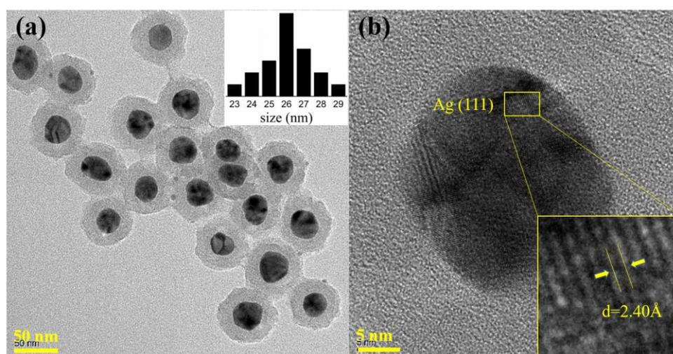
**Figure 1.** (a) TEM image and size distribution results of Ag@SiO<sub>2</sub> NPs; (b) HRTEM image of a Ag@SiO<sub>2</sub> NP.
