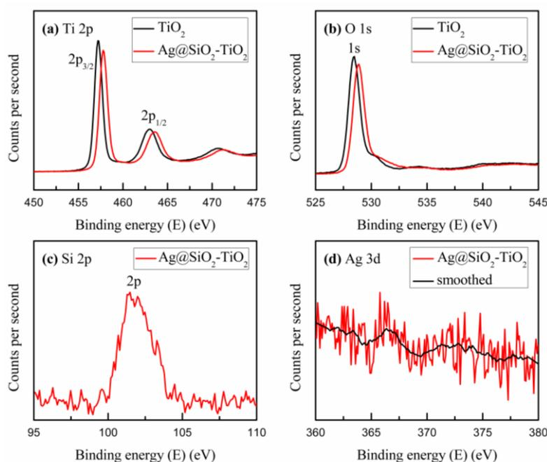
**Figure 3.** XPS survey spectra acquired from mesoporous TiO<sub>2</sub> and the Ag@SiO<sub>2</sub>-TiO<sub>2</sub>: (a) Ti 2p; (b) O 1s; (c) Si 2p; (d) Ag 3d.
