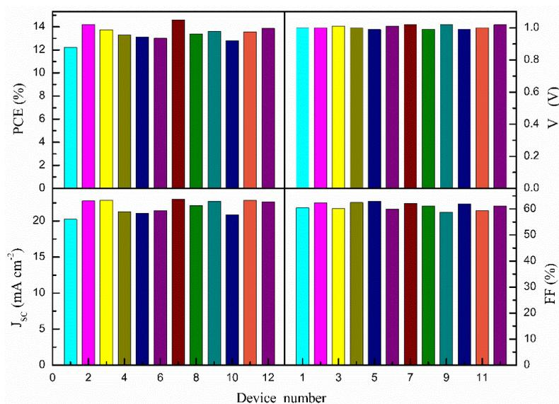
**Figure 7.** Histograms of photovoltaic parameters for 12 devices (the same batch of samples) based on mesoporous  $\text{TiO}_2$  film mixed with 0.3 wt. %  $\text{Ag@SiO}_2$  NPs.
