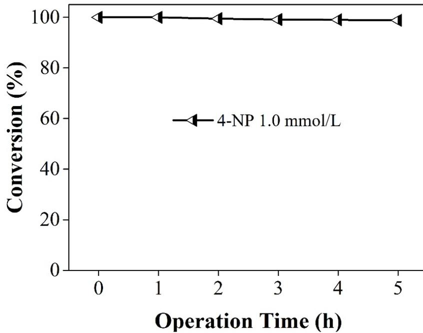
**Figure S5.** Effect of operation time on the catalytic performance of an Au/N-rGO (Au/C=0.2%) membrane.
