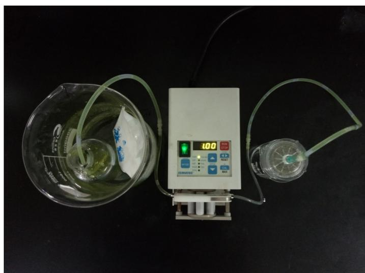
**Figure S1.** The photograph of operational device in flow catalytic system.
