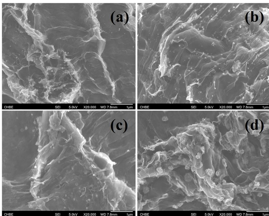
**Figure S2.** Field emission scanning electron microscopy (FESEM) images of gold/nitrogen-doped graphene (Au/N-rGO) composites with different Au loading amounts. Au/C ratio is (a) 0.5%, (b) 1.0%, (c) 2.0%, and (d) 5.0%, respectively.
