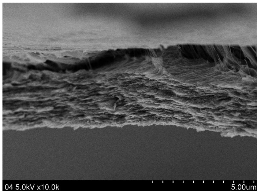
**Figure S3.** FESEM images for cross sectional analysis of Au/N-rGO filter.
