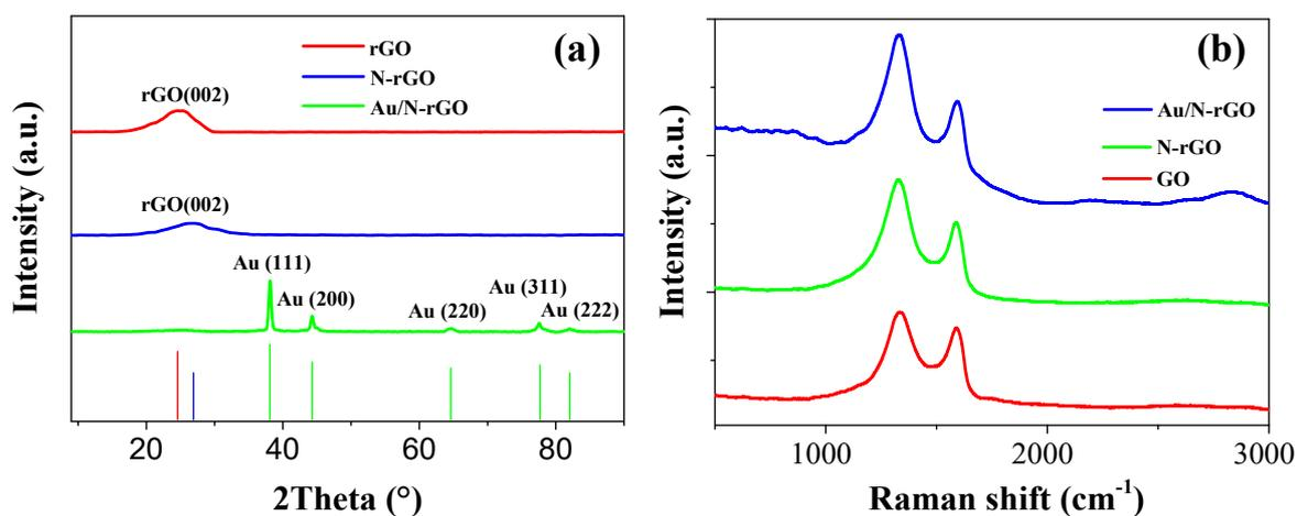
**Figure S4.** XRD diffraction patterns of pure rGO, pure N-rGO and Au/N-rGO filters (a); Raman spectra recorded from GO, N-rGO and Au/N-rGO (Au/C=0.2%) samples (b).
