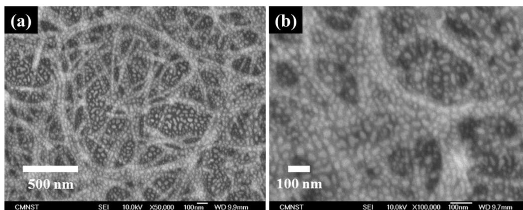
Supporting Data 1: (a) Low magnification and (b) high magnification of FE-SEM images for the sample AuNPs/ZrO<sub>2</sub>NFs<sub>0.3</sub>. A uniform Au NPs are deposited onto ZrO<sub>2</sub> NFs.
