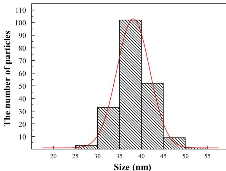
Supporting Data 3: The size distribution histogram of Au NPs on the sample AuNPs/ZrO<sub>2</sub>NFs\_0.3. To calculate the sizes, random 200 particles on the Supporting Data 1(a) are chosen.
