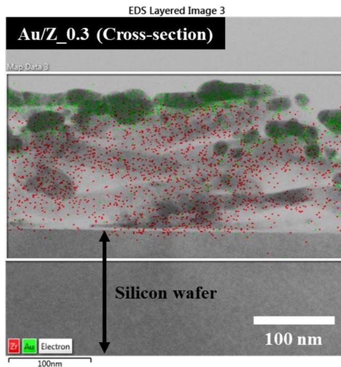
Supporting Data 2: The EDS-mapping image of the cross-sectioned sample AuNPs/ZrO<sub>2</sub>NFs\_0.3. The green spot is Au element, while the red spot is Zr one.
