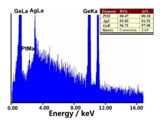
Figure S2. The EDS spectra of the the Ge wafer grown with Ag-Pt nanoparticles.
