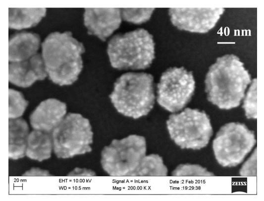
Figure S1. The high magnification SEM images of Ag-Pt nanoparticles grafted on the Ge wafer.
