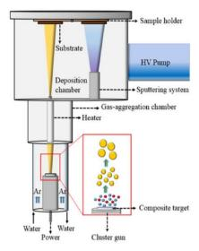
**Figure 1.** Fabrication of Mn<sub>5</sub>Ge<sub>3</sub> nanoparticles. A schematic illustration of the cluster-beam-deposition (CBD) process.
