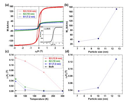
**Figure 7.** Magnetization and extrinsic magnetic properties of the nanoparticles: (a) hysteresis loops measured at 50 K; (b) saturation magnetization versus particle size; (c) coercivity versus temperature; and (d) coercivity versus particle size.
