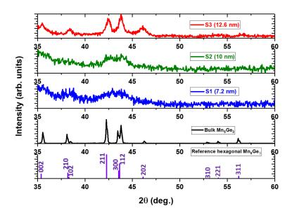
**Figure 2.** X-ray diffraction (XRD) patterns for the reference  $Mn_5Si_3$ -type hexagonal crystal structure, for the bulk  $Mn_5Ge_3$  and for the samples S1, S2, and S3.
