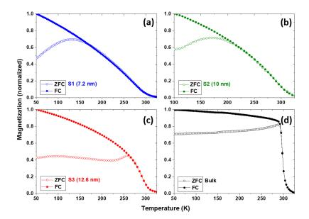
**Figure 6.** Temperature-dependent magnetization curves of the samples (a) S1; (b) S2; (c) S3; and (d) powdered bulk measured at 0.05 T.
