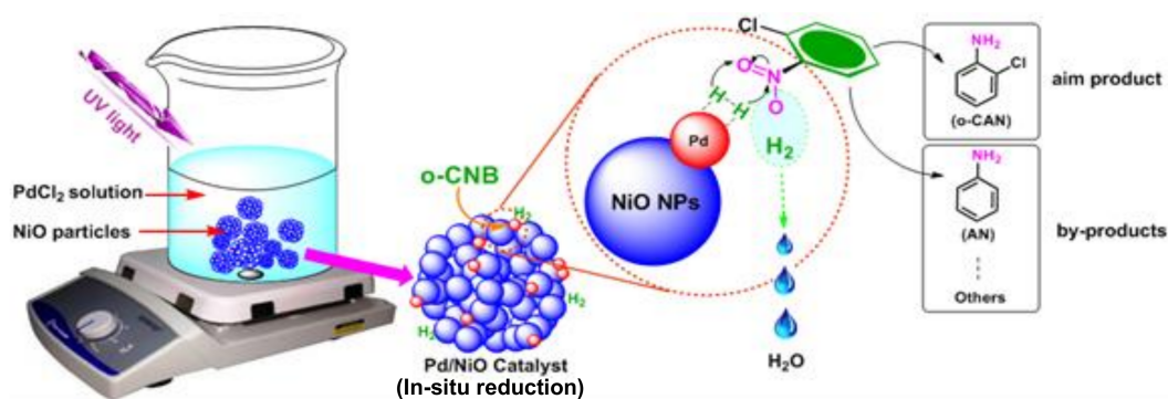
Scheme 1. Sketch map of the preparation of UV-light-irradiated Pd-based catalyst over NiO and the evaluation of its reactivity toward the o -chloronitrobenzene ( o -CNB) hydrogenation.
